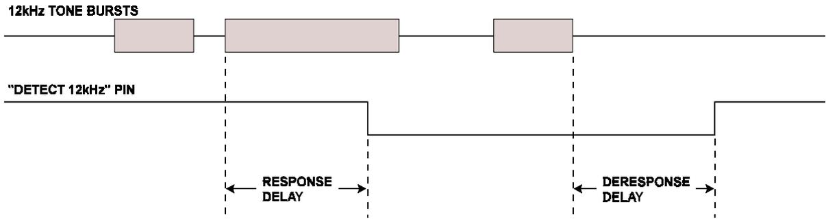
(a) SPM (12kHz) channel. Toneburst and tonegaps less than the response and de-response delays are ignored.
