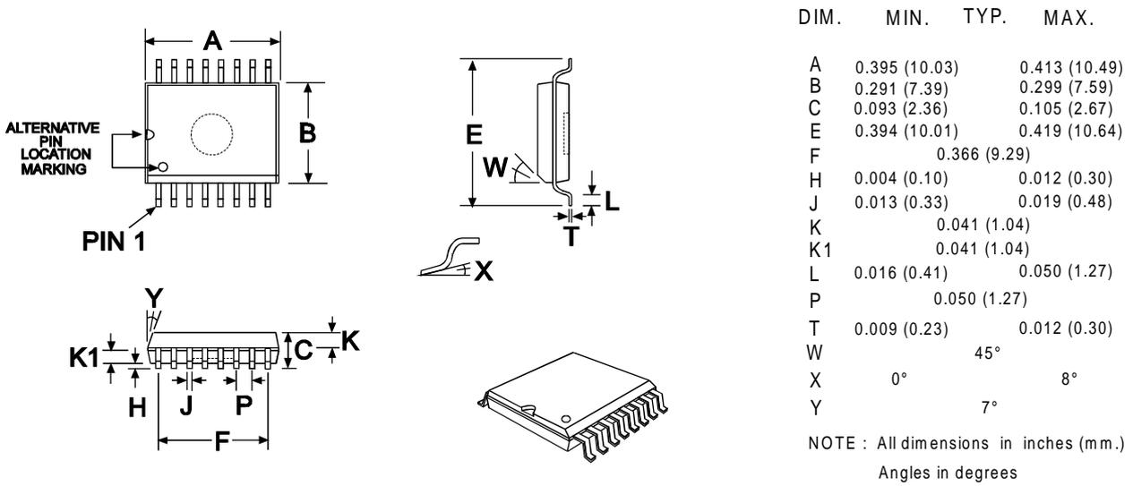
**Figure 4 SOIC Mechanical Outline: Order as part no. FX651D4**
