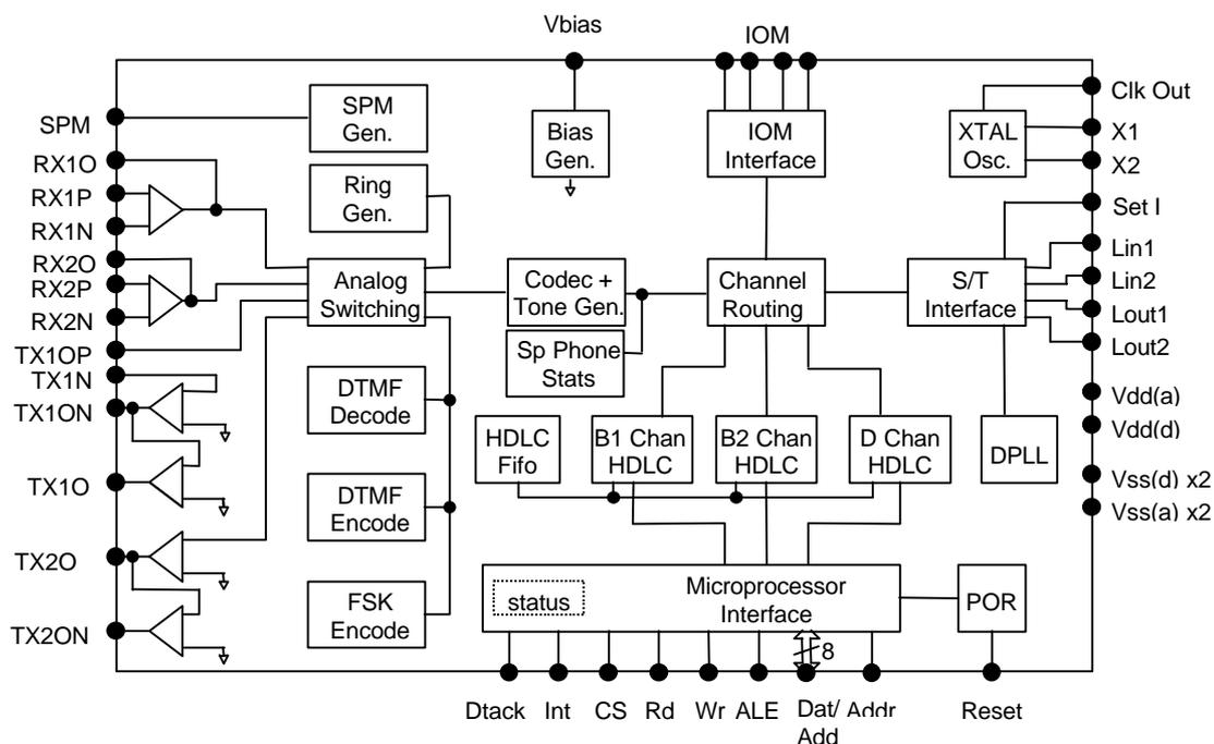
RX1 and RX2 channels used for Mic or POTS input.
