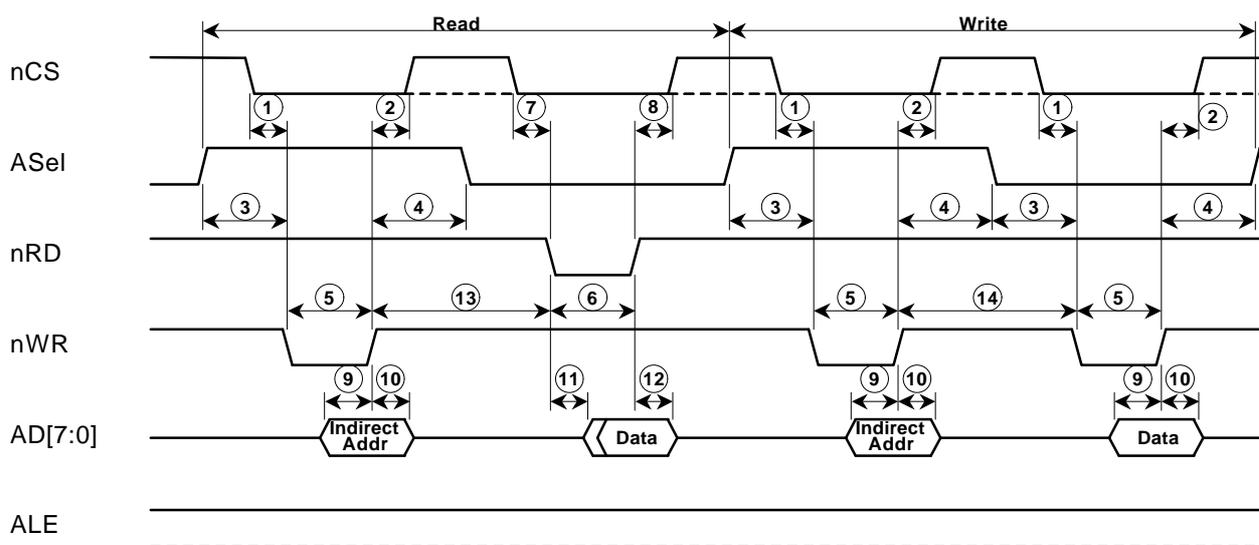
Figure 24. Processor Bus Timing – Intel Non-multiplexed
