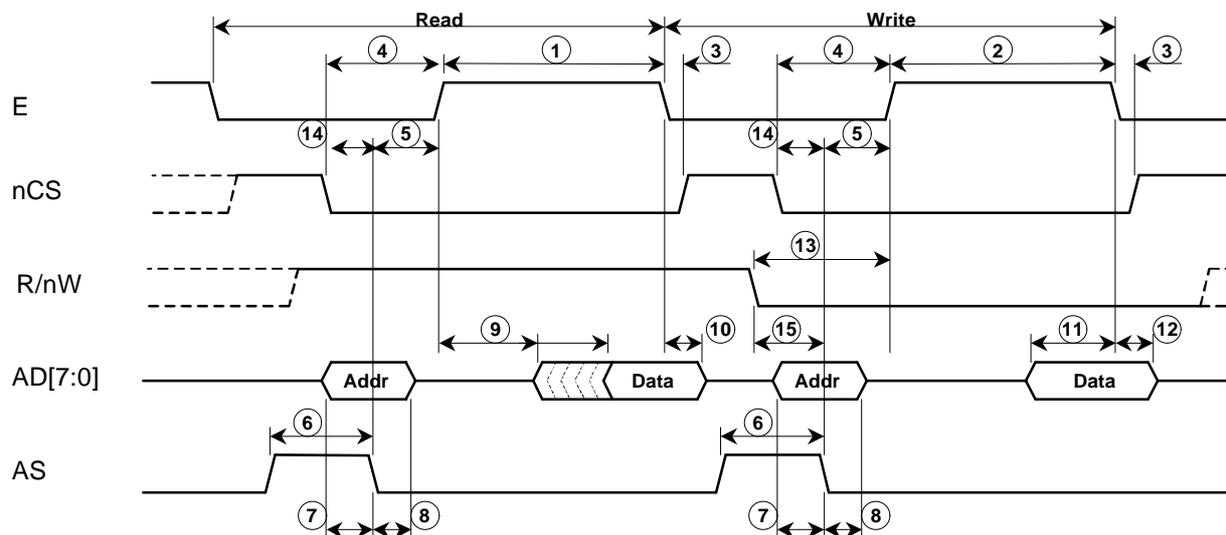
Figure 23. Processor Bus Timing – Motorola Multiplexed
