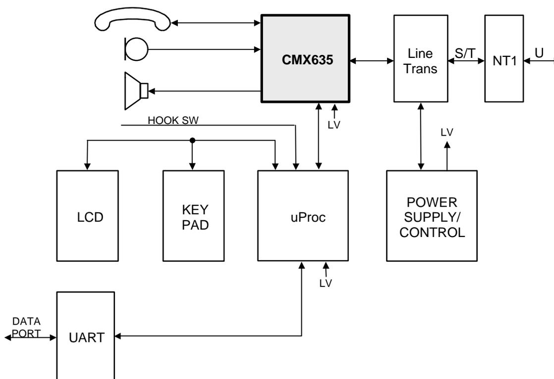
**Figure 9. ISDN Telephone Configuration**
