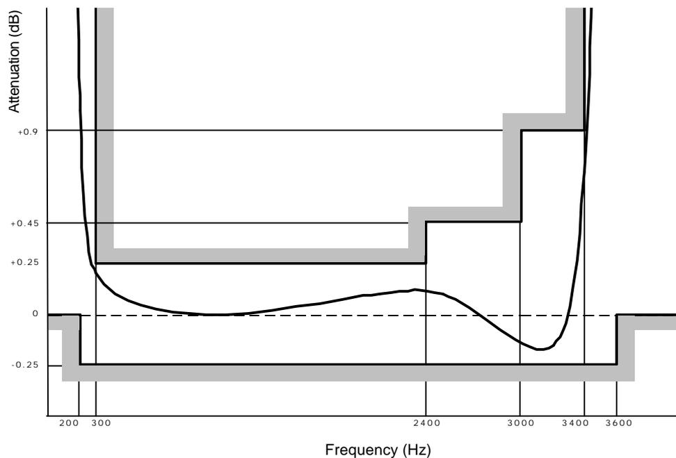
**Figure 20. Codec Filter Attenuation Characteristics and Limits**
