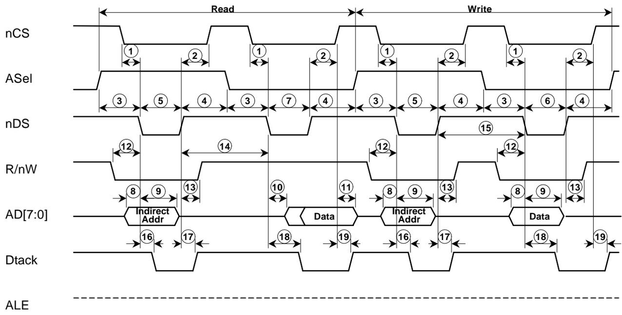
Figure 26. Processor Bus Timing – Motorola Non-multiplexed
