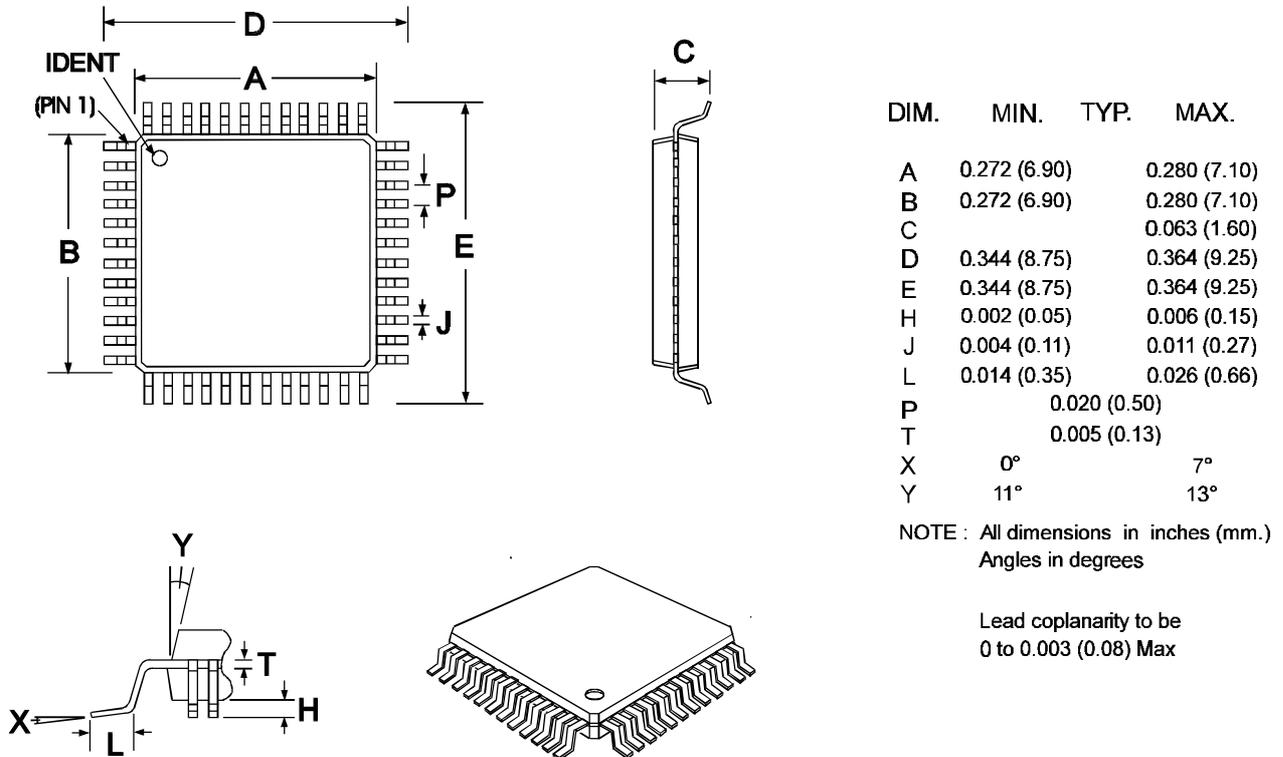
Figure 28. 48-Pin TQFP (L4) Mechanical Outline
