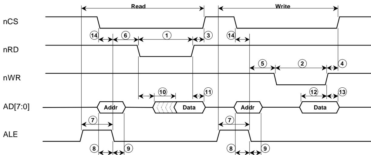
**Figure 22. Processor Bus Timing – Intel Multiplexed**
