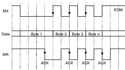
**Figure 16. Monitor Handshake Timing (maximum speed case)**
