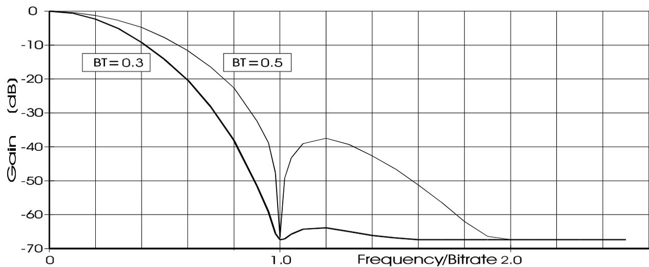
Figure 6 Tx Output Baseband Spectrum (for random data)
