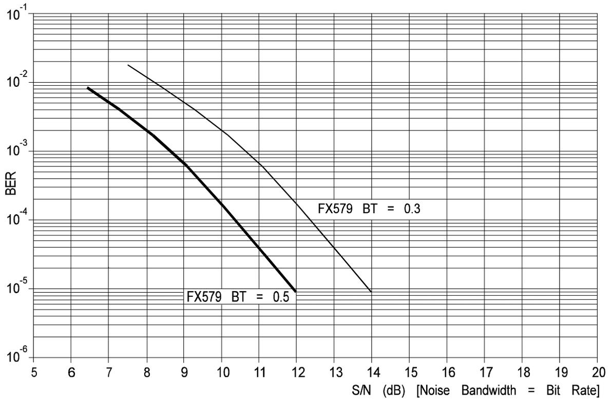
Figure 9 Typical Bit Error Rate Performance
