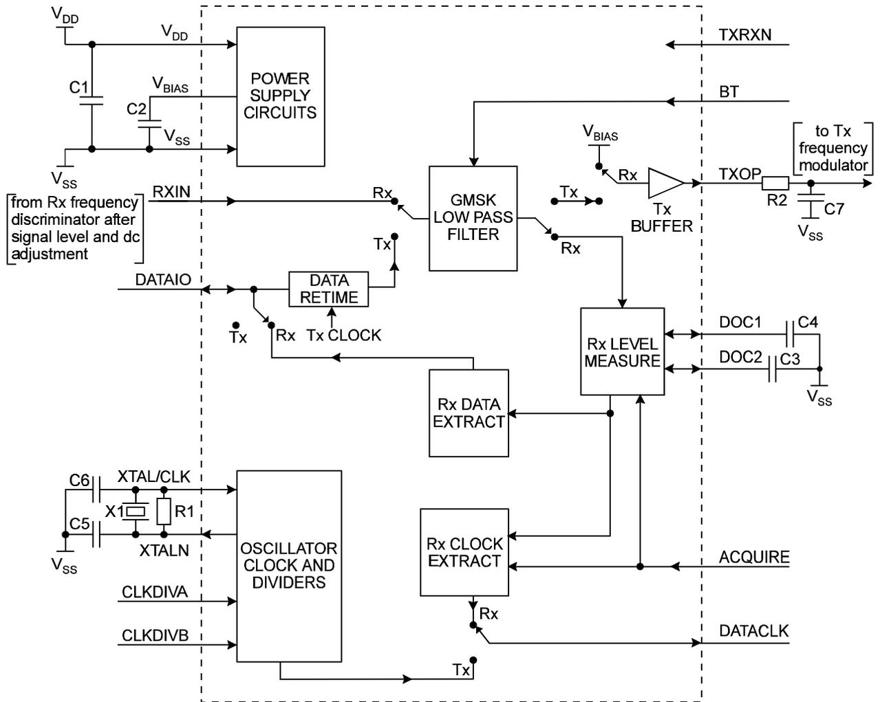
Figure 1 Block Diagram
