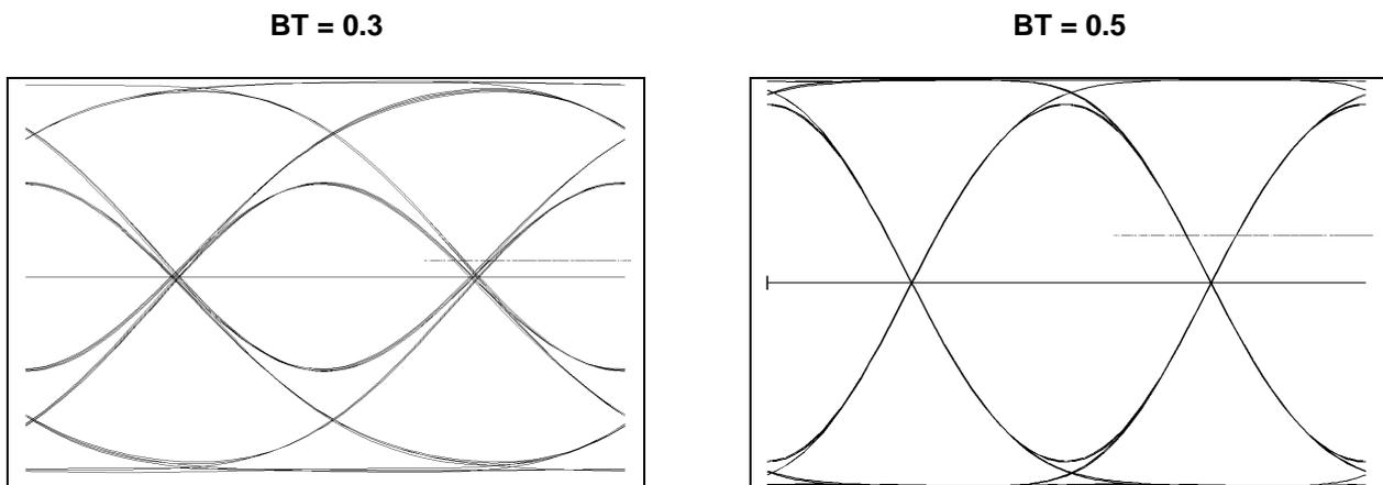
Figure 5 Typical Transmit Eye Patterns (after external RC network)
