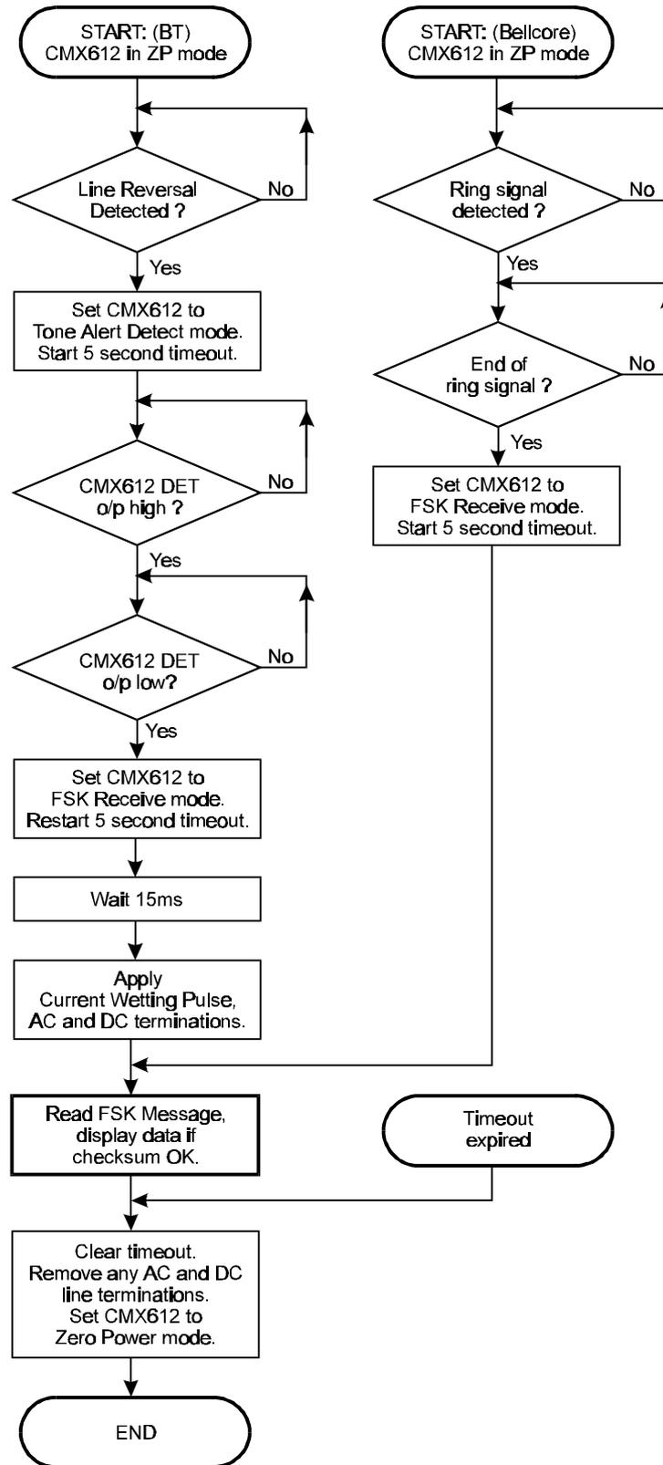
Figure 9c : Flow Chart for On-hook operation of CMX612
