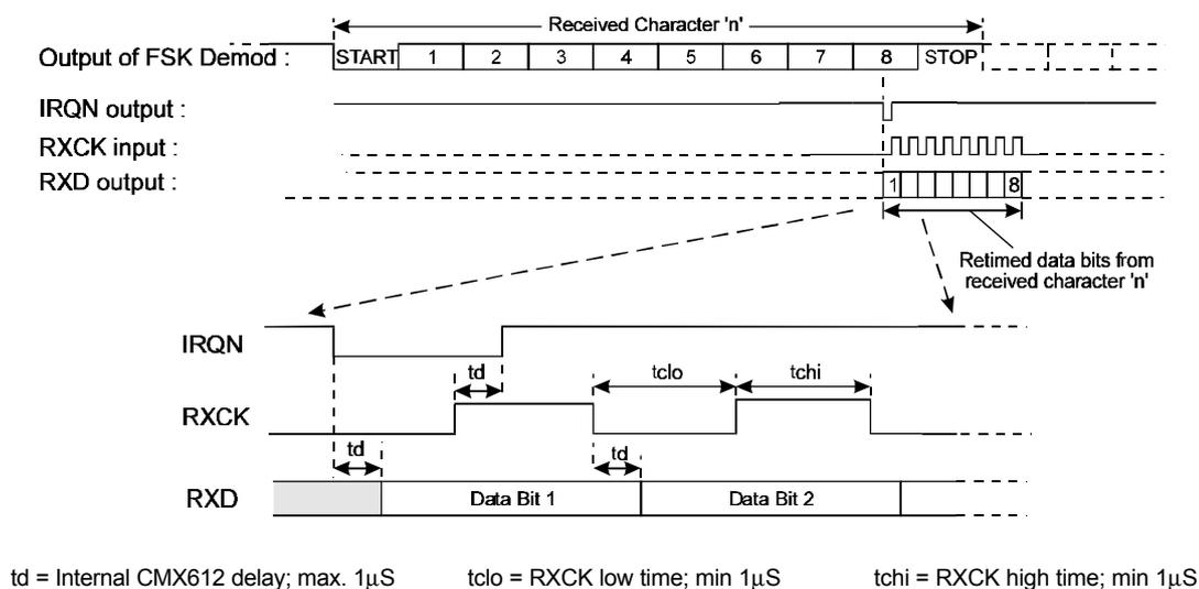
**Figure 5a : FSK Operation With Data Retiming**
