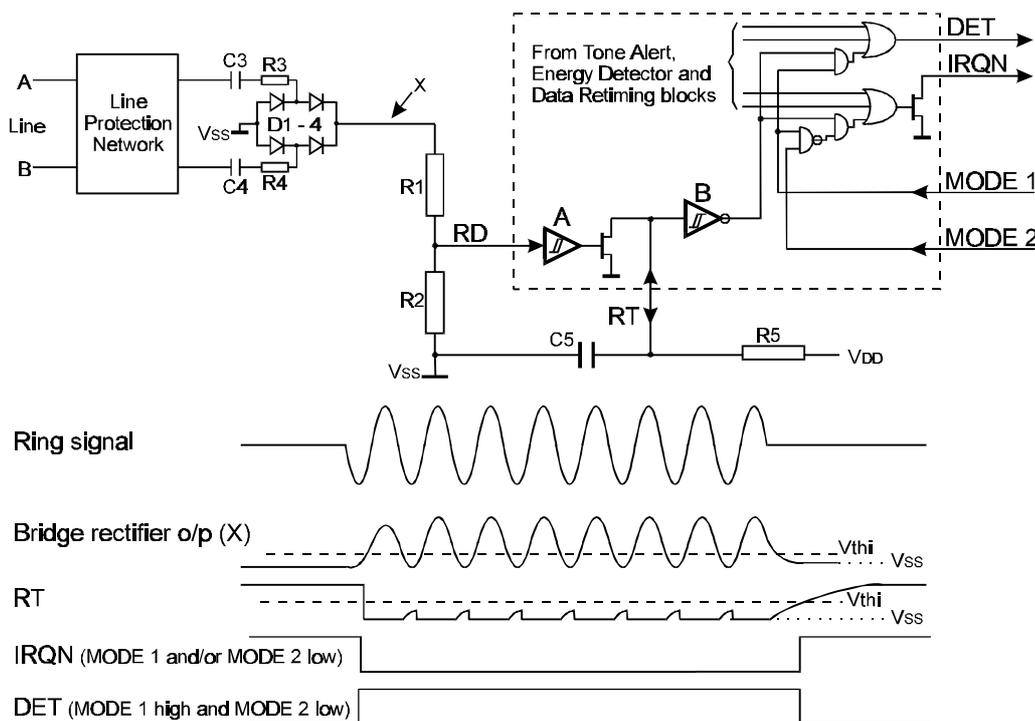
Figure 8 : Ring or Line Polarity Reversal operation
