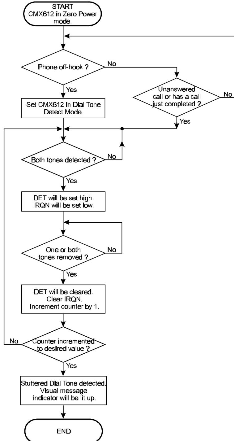
Figure 11 : Flow Chart for VMWI-SDT operation of CMX612
