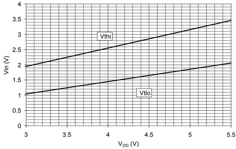
Figure 12 : Schmitt Trigger typical input voltage thresholds vs. V<sub>DD</sub>
