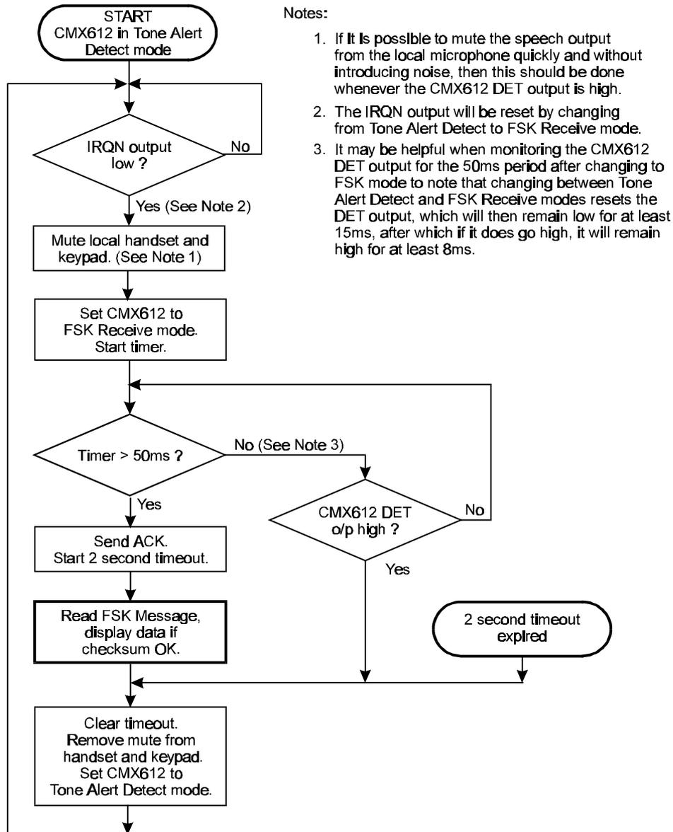
Figure 10b : Flow Chart for Off-hook operation of CMX612
