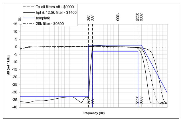
Figure 9 Tx Channel Audio Filter Response and Template (TIA)
