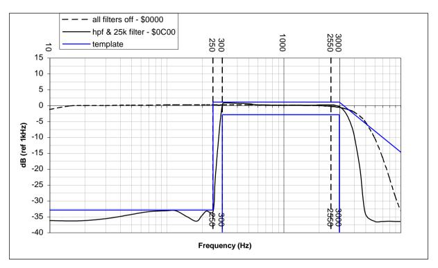
Figure 6 Rx 25kHz Channel Audio Filter Frequency Response
