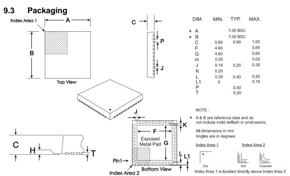
Depending on the method of lead termination at the edge of the package, pull back (L1) may be present. L minus L1 to be equal to, or greater than 0.3mm The underside of the package has an exposed metal pad which should ideally be soldered to the pcb to enhance the thermal conductivity and mechanical strength of the package fixing. Where advised, an electrical connection to this metal pad may also be required
