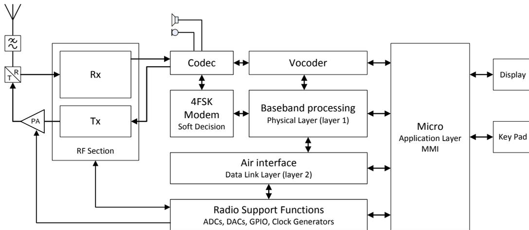
Figure 1: Typical Digital Radio Function Block Diagram
