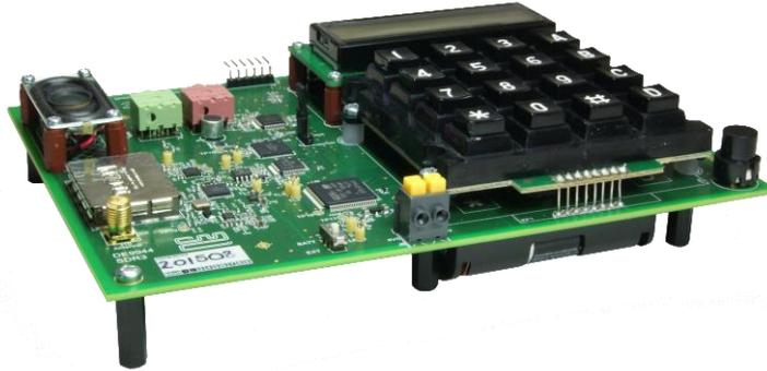
Figure 3: DE9944 SDR FDMA Radio demonstrator
