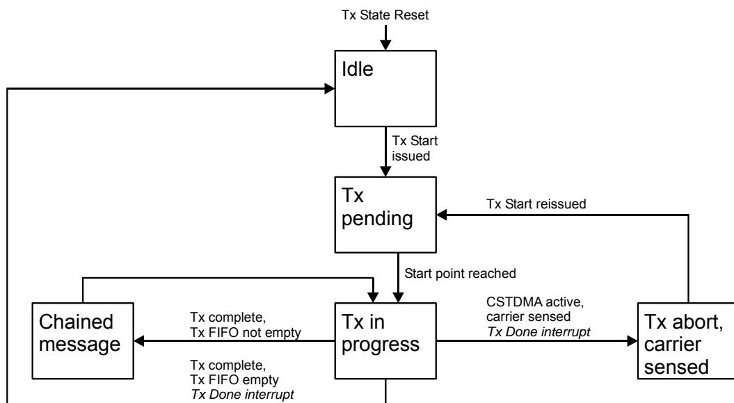
**Figure 7 Tx (AIS raw mode) state transitions**
