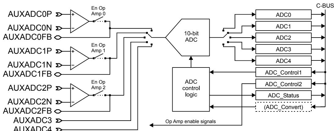
**Figure 12 Auxiliary ADC**
