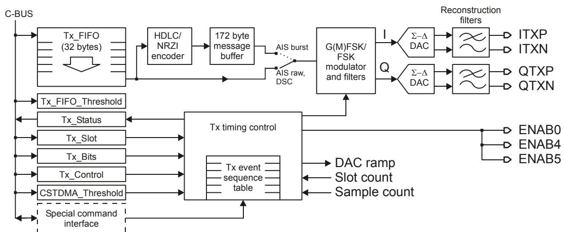
**Figure 6 Transmit Channel**
