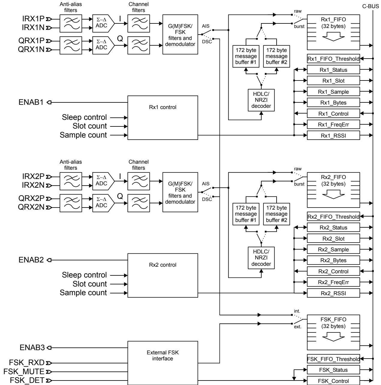
Figure 11 Receive Channel
