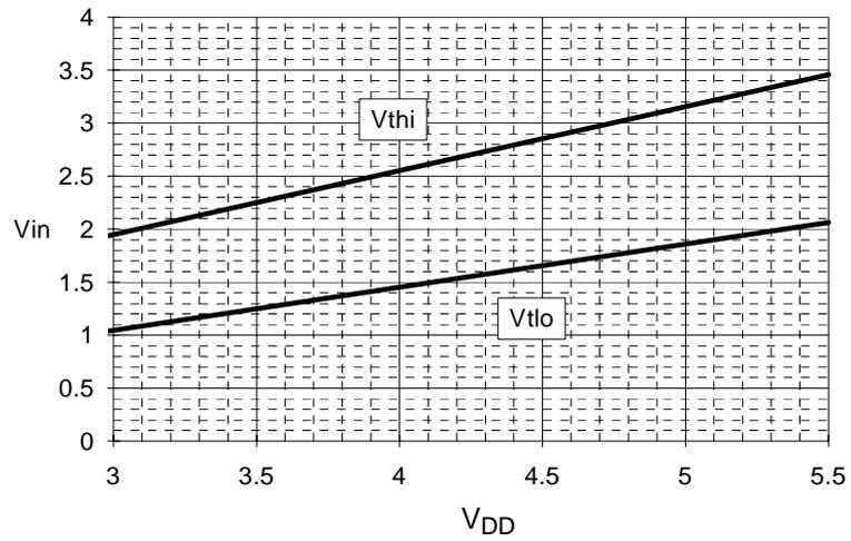
Figure 10 : Schmitt Trigger typical input voltage thresholds vs. V<sub>DD</sub>
