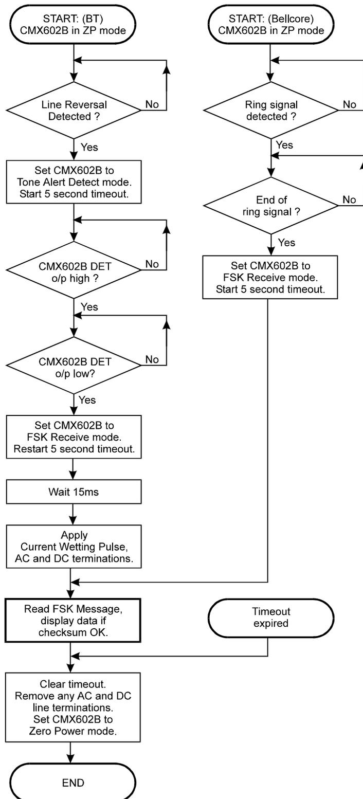
Figure 8c : Flow Chart for On-hook Operation of CMX602B
