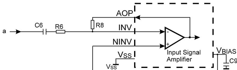
**Figure 3b : Input Signal Amplifier, unbalanced input configuration**
