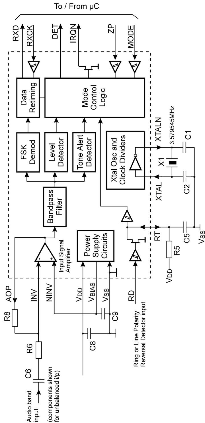
Figure 1 Block Diagram
