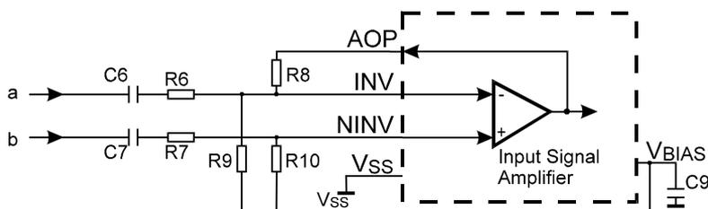
Figure 3a : Input Signal Amplifier, balanced input configuration
