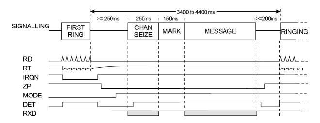
Figure 8b : Bellcore On-hook System Signals
