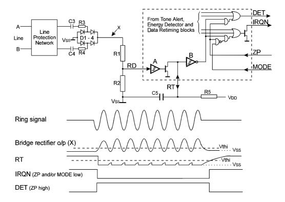
Figure 7: Ring or Line Polarity Reversal operation
