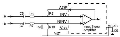
Figure 3a: Input Signal Amplifier, balanced input configuration
