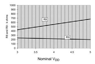
Figure 3c : Input Signal Amplifier, optimum values of R8 and R9 vs V<sub>DD</sub>
