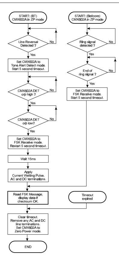
Figure 8c: Flow Chart for On-hook Operation of CMX602A
