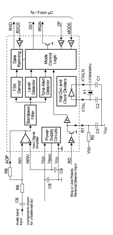
Figure 1 Block Diagram
