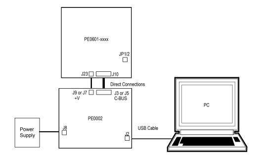
Figure 2 – PE0601 used with PE0002
