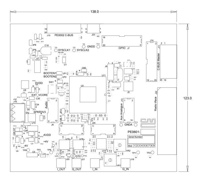
Figure 3 - PCB Layout: Top
