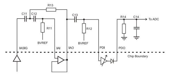
Figure 6 Typical Instability Detector Section Configuration
