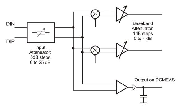
Figure 12 Downconverter Attenuation Configuration and RF Detector
