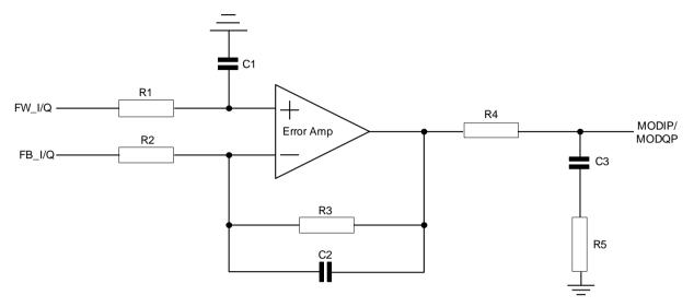
Figure 7 Error Amplifier External Component Configuration
