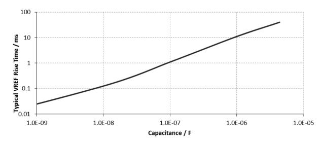
Figure 11 – Typical Rise Time of Reference Voltage
