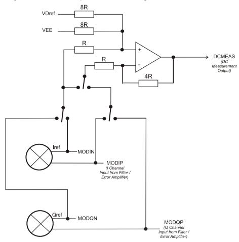
Figure 9 Configuration of DCMEAS output switching
