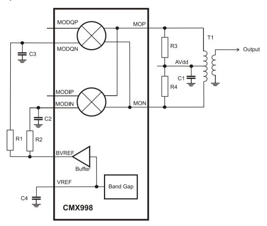
Figure 3 Modulator and Bias External Components
