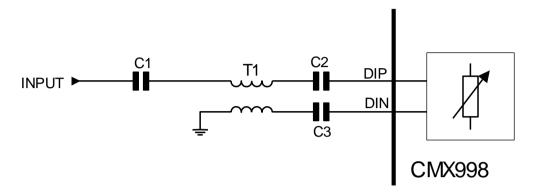
Figure 4 Downconverter External Component Configuration
