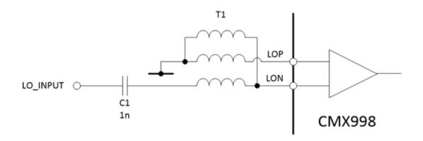
Figure 5 LO Input Configuration using a 1:1 Balun
