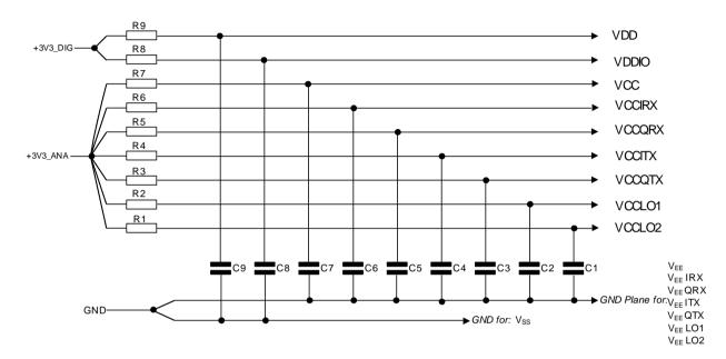
Figure 2 Power Supply Connections and Decoupling
