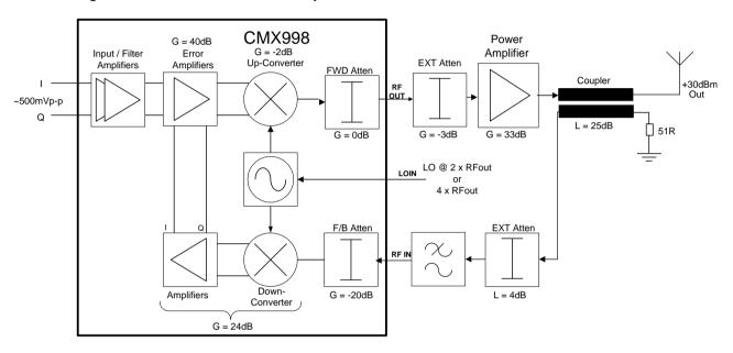
Figure 8 Typical Cartesian Loop Configuration using the CMX998
