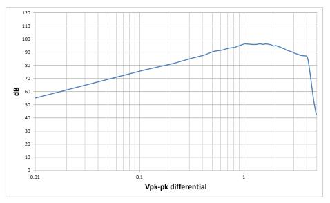
Figure 36 Main ADC SFDR vs. Input Level - WBM
