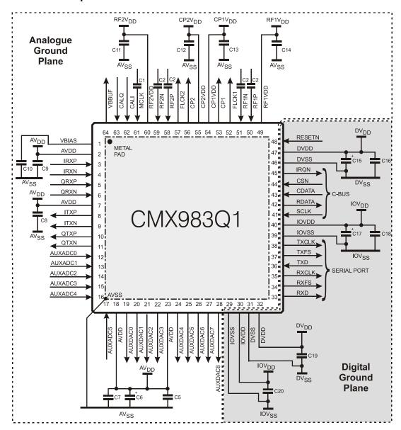
Figure 3 Recommended External Components - General
