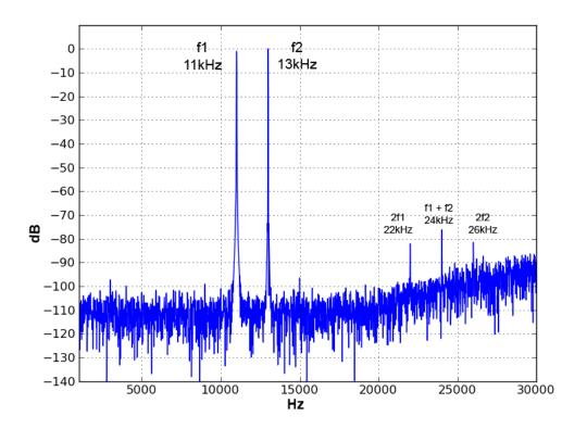
Figure 37 Main ADC Two Tone Test - NBM
