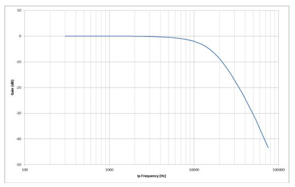
Figure 51 DAC Frequency Response (Σ-Δ clock=2.4MHz, SC Filter Bandwidth=Low)
