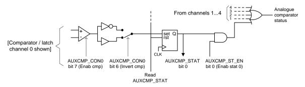
Figure 27 Comparator and Threshold Status Flag
