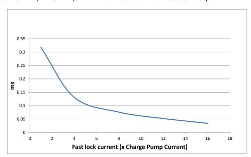
Figure 47 PLL2 Indicated Lock Time vs. Fast Lock Current (2125 to 2043 MHz)
