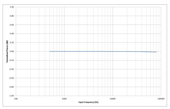
Figure 50 ADC Modulator Frequency Response (Σ-Δ clock=4.8MHz)
