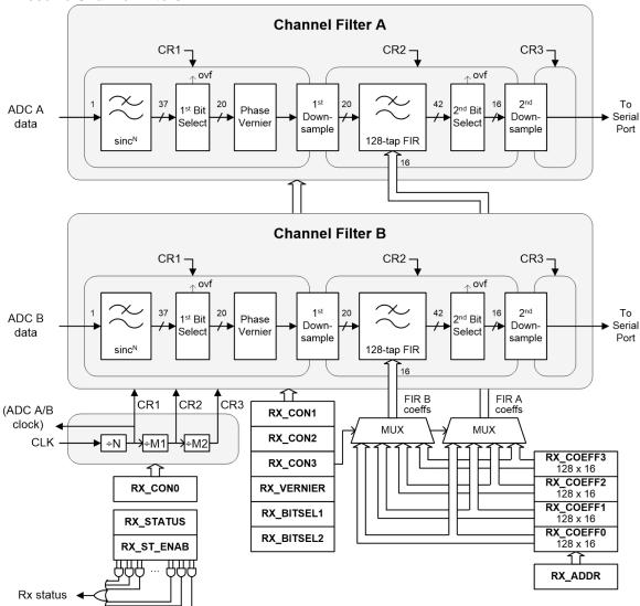
Figure 13 Rx Channel Filters
