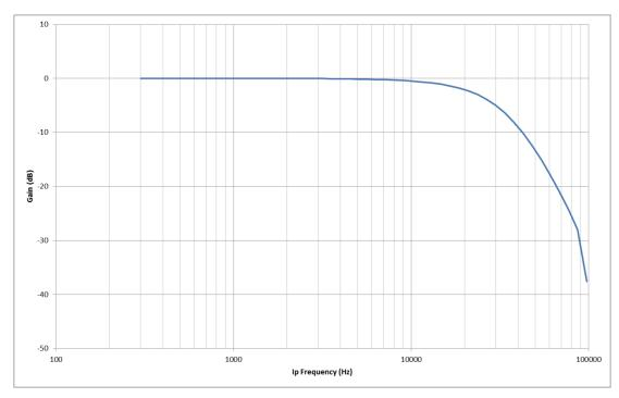
Figure 53 DAC Frequency Response (Σ-Δ clock=4.8MHz, SC Filter Bandwidth=Low)
