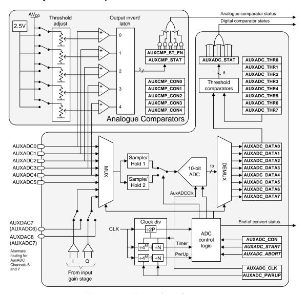
Figure 25 Auxiliary ADC and Comparators
