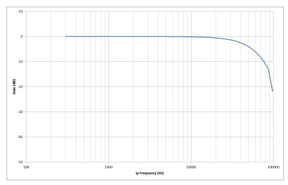
Figure 54 DAC Frequency Response (Σ-Δ clock=4.8MHz, SC Filter Bandwidth=High)
