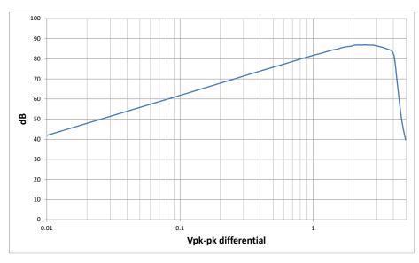
Figure 35 Main ADC SINAD vs. Input Level - WBM
