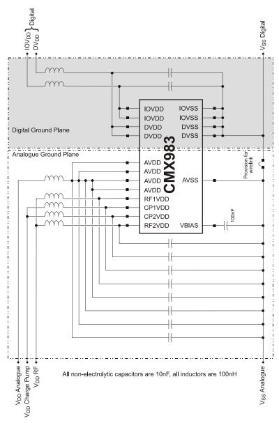
Figure 4 Power Supply Decoupling
