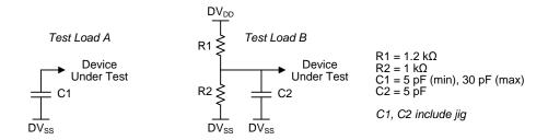
Figure 30 AC Test Load for Digital Outputs
