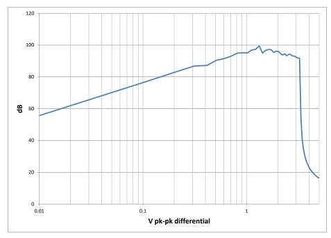
Figure 34 Main ADC SFDR vs. Input Level - NBM
