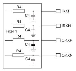
Figure 5 Recommended External Components - Rx Inputs
