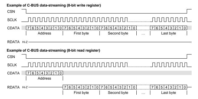
Figure 8 C-BUS Data-streaming Operation
