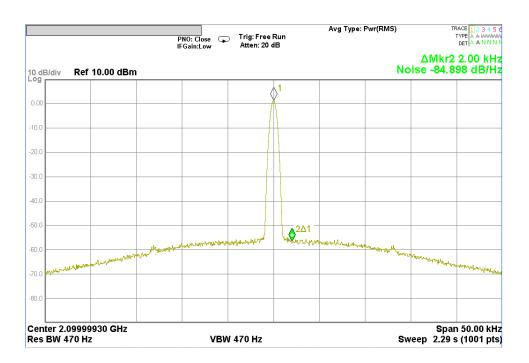
Figure 45 PLL2 Output Spectra
