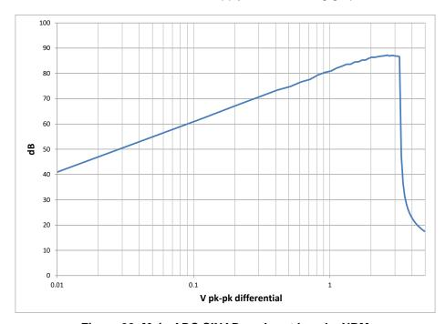
Figure 33 Main ADC SINAD vs. Input Level - NBM
