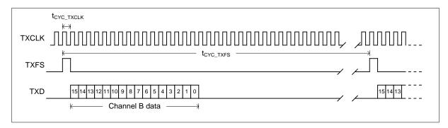
Figure 20 Tx Port Timing (Channel B only selected)
