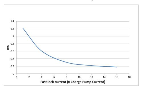
Figure 44 PLL1 Indicated Lock Time vs. Fast Lock Current (965 to 875.525 MHz)
