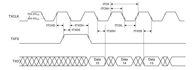
Figure 32 Serial Port Timings
