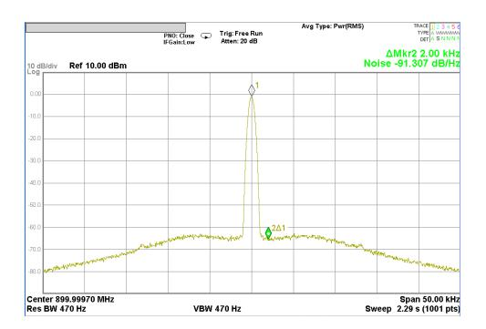
Figure 42 PLL1 Output Spectra
