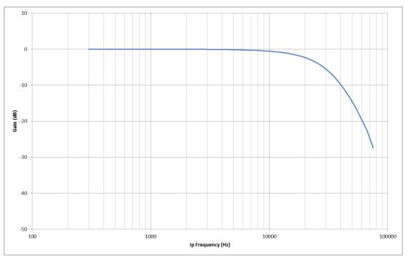
Figure 52 DAC Frequency Response (Σ-Δ clock=2.4MHz, SC Filter Bandwidth=High)
