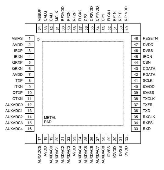
The exposed metal pad at the underside of the package must connect to AVSS
