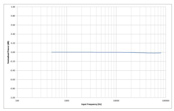
Figure 49 ADC Modulator Frequency Response ( $\Sigma$ - $\Delta$  clock=2.4MHz)
