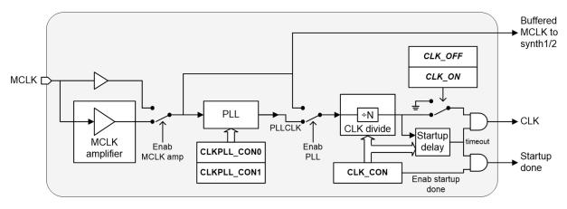
Figure 11 System Clock Generator
