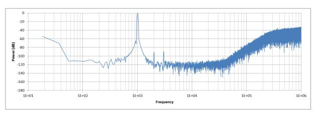
Figure 56 ADC Modulator Spectrum (Clock Rate = 4.8MHz)
