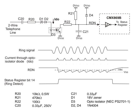
Resistors ±5%, capacitors ±20%. Typical circuit, component types and values.
