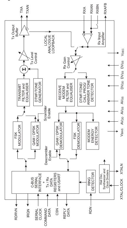
Figure 1 Block Diagram
