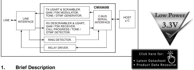
The CMX869B is a multi-standard modem for use in EPOS terminals and telephone based information and telemetry systems. This highly integrated single-chip modem IC provides the functions needed to construct a ITU V.32 bis automode modem or a V.22 bis, V.22, V.21 and Bell 202, Bell 103 compatible modem operating under the control of external host timing for EPOS and other proprietary protocols.
