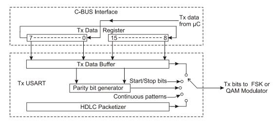
Figure 5c Tx USART (in 16 Bit Mode)
