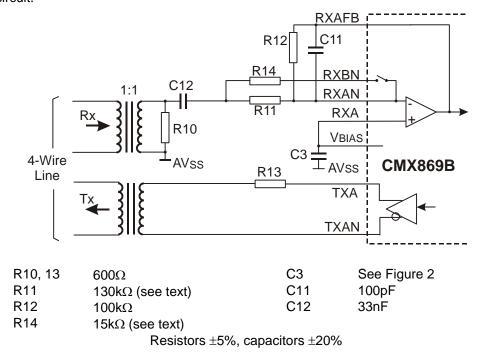
Figure 4b 4-Wire Line Interface Circuit
