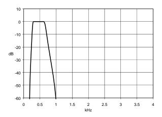
Figure 6 Response of Call Progress Filter
