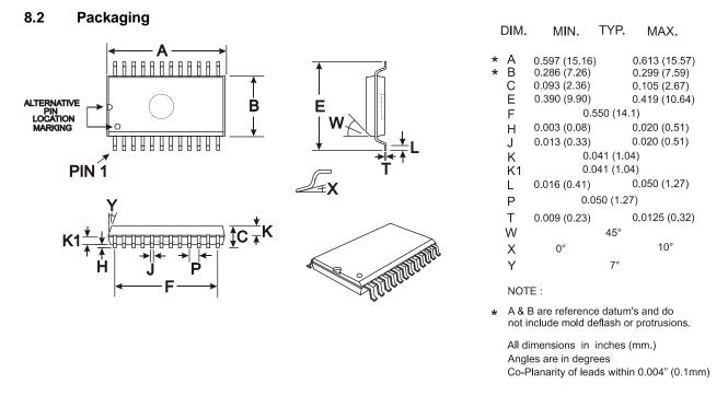
Figure 14a 24-pin SOIC (D2) Mechanical Outline: Order as part no. CMX869BD2
