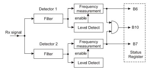
Figure 10a Programmable Tone Pair Detector
