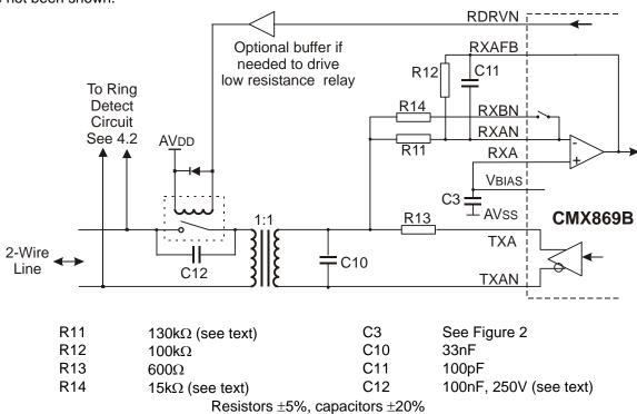
Figure 4a 2-Wire Line Interface Circuit
