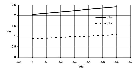
Figure 11 Typical Schmitt Trigger Input Voltage Thresholds vs. V<sub>DD</sub>
