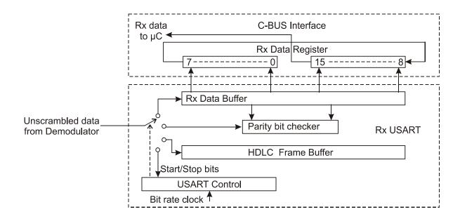
Figure 7 Rx USART (in 16-bit Mode)
