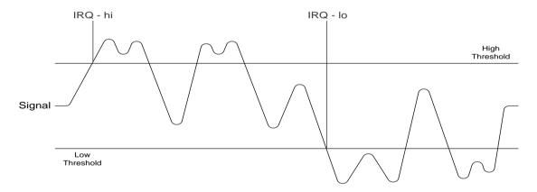
Figure 31 AuxADC IRQ Operation
