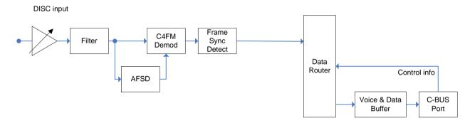
Figure 14 Internal C4FM Data Processing Blocks
