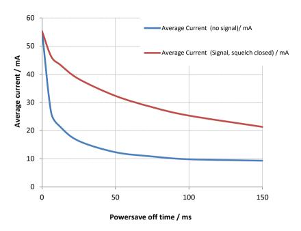
Figure 25 Effect of Powersave as a Function of "OFF" Time (Best and Worst Case)
