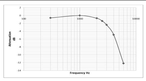
Figure 20 Frequency Response for Rx Pass-through Mode
