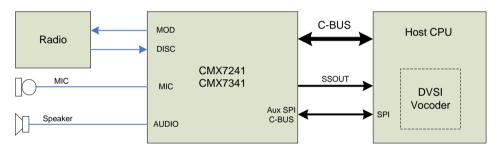
Figure 8 DVSI Vocoder Connection
