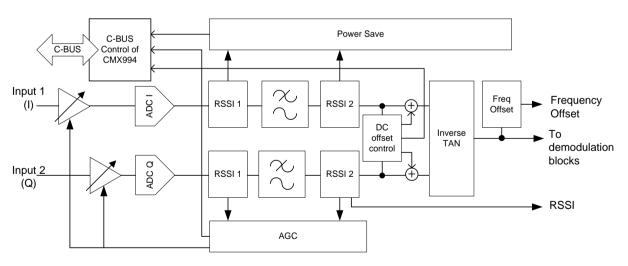
Figure 15 Additional Internal Data Processing in I/Q Mode
