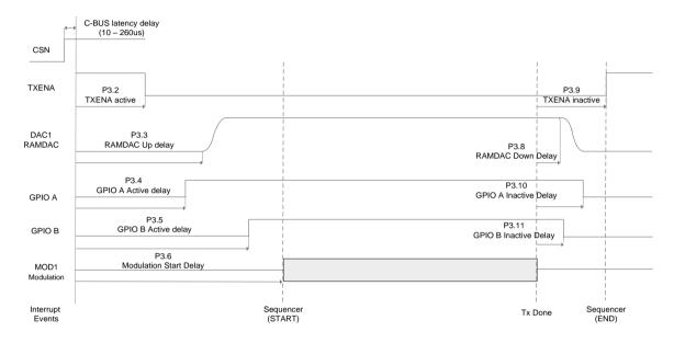
Figure 19 Tx Sequencer Delay Timers
