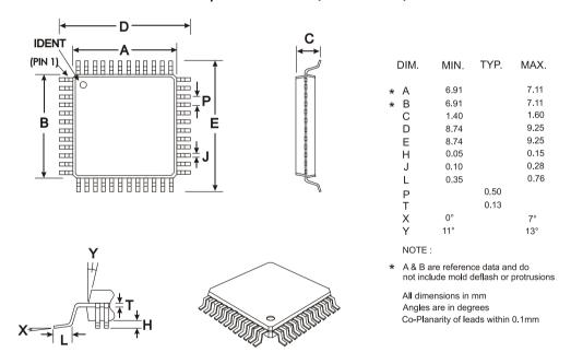
Figure 38 Mechanical Outline of 48-pin LQFP (L4)
