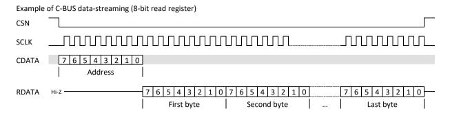
Figure 17 C-BUS Data-Streaming Operation
