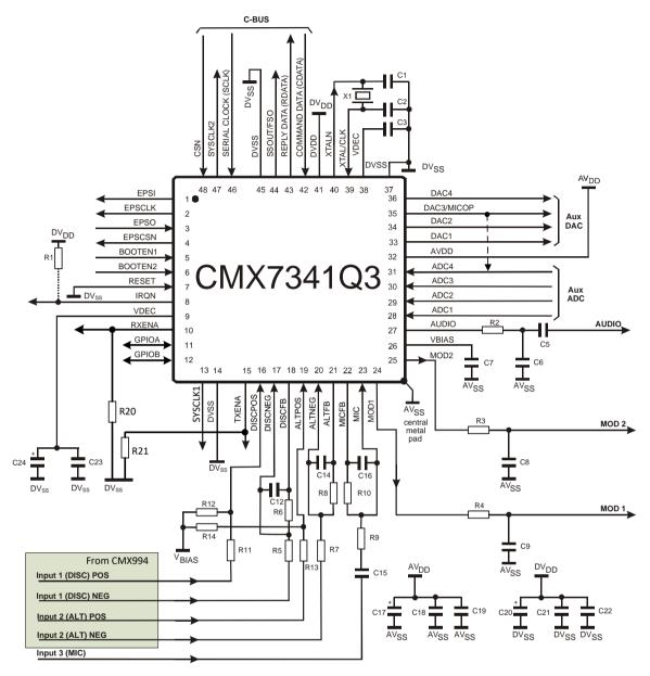
Figure 3 CMX7341 (Q3) Recommended External Components
