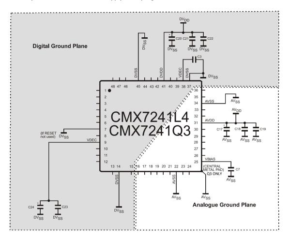
Figure 4 CMX7241 (L4/Q3) Power Supply and Decoupling
