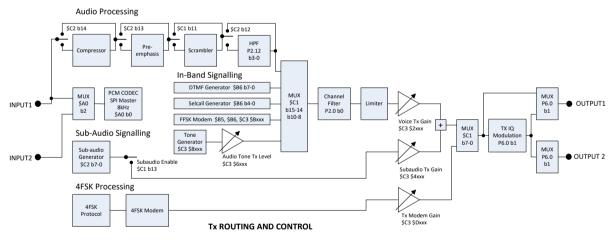
Figure 26 Rx and Tx Level Adjustments and Routing
