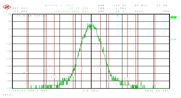
Figure 15 4FSK PRBS Waveform - Spectrum
