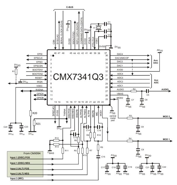
Figure 3 CMX7341 (Q3) Recommended External Components
