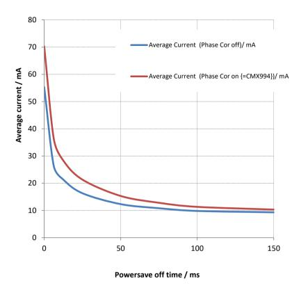
Figure 29 Effect of Powersave as a Function of "OFF" Time
