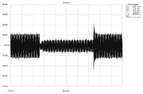
Figure 36 Compressor Transient Response
