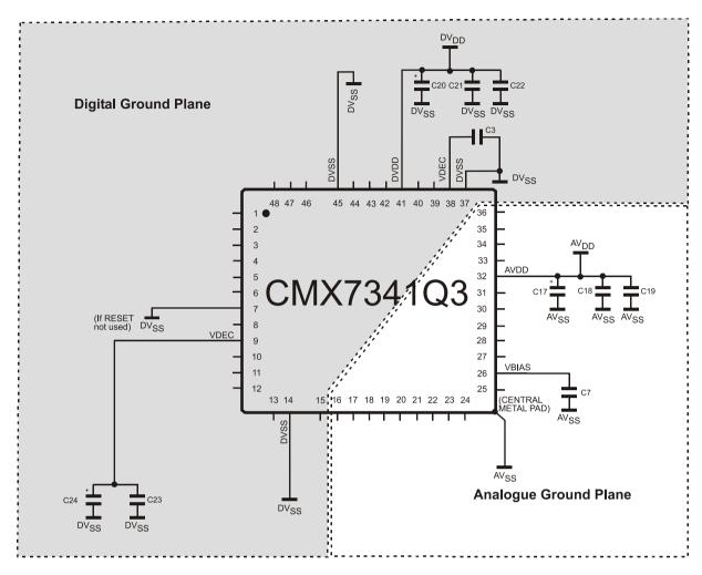
Figure 5 CMX7341 (Q3) Power Supply and De-coupling
