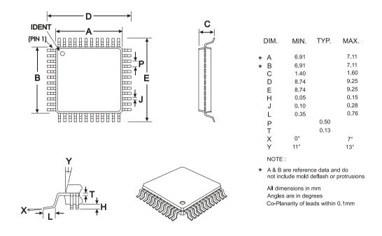
Figure 49 Mechanical Outline of 48-pin LQFP (L4)
