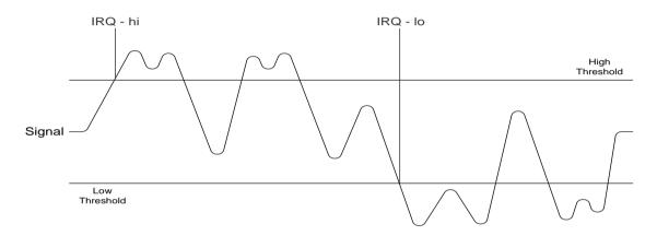
Figure 42 AuxADC IRQ Operation
