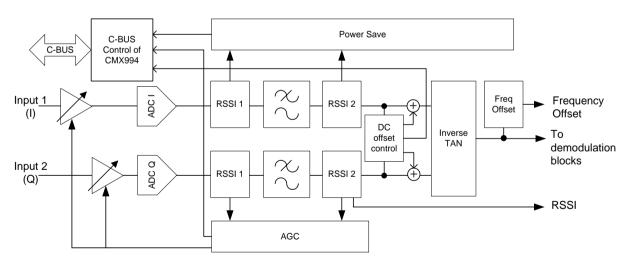
Figure 18 Additional Internal Data Processing in I/Q Mode
