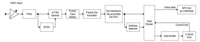
Figure 17 Internal 4FSK Data Processing Blocks
