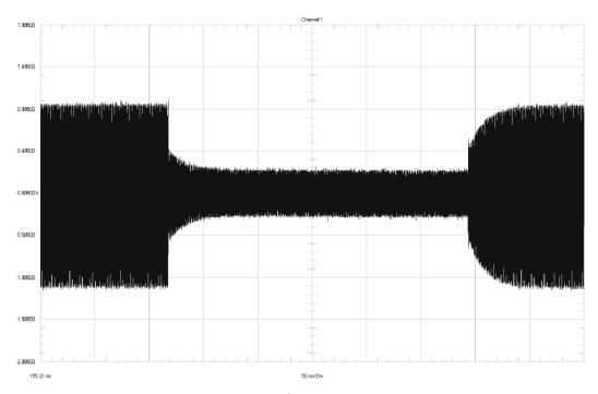
Figure 35 Expandor Transient Response
