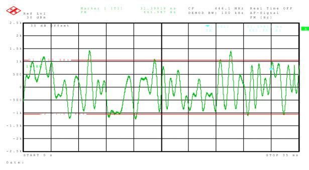
Figure 14 4FSK PRBS Waveform - Modulation
