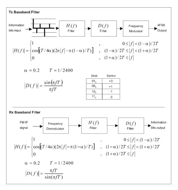
Figure 16 4FSK Modulation Characteristics
