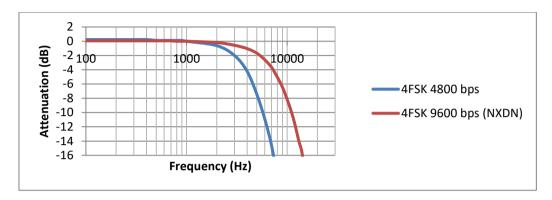
Figure 25 Frequency Response for Rx Pass-through Mode
