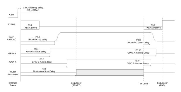
Figure 24 Tx Sequencer Delay Timers
