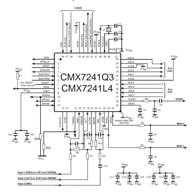
Figure 2 CMX7241 (L4 and Q3) Recommended External Components
