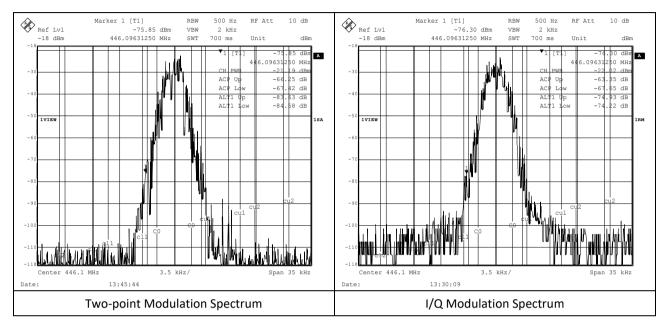
Figure 46 Tx Modulation Spectra – 4.8kbps
