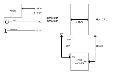
Figure 11 DVSI Vocoder Connection
