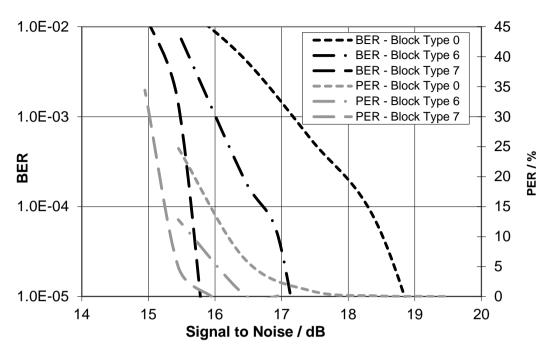
Figure 100 Comparison of BER and PER for 32-QAM Modulation
