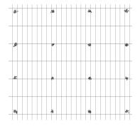
Figure 32 Normalised Constellation (even with a frequency or phase error)
