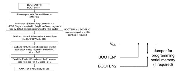
Figure 16 FI Loading from Serial Memory
