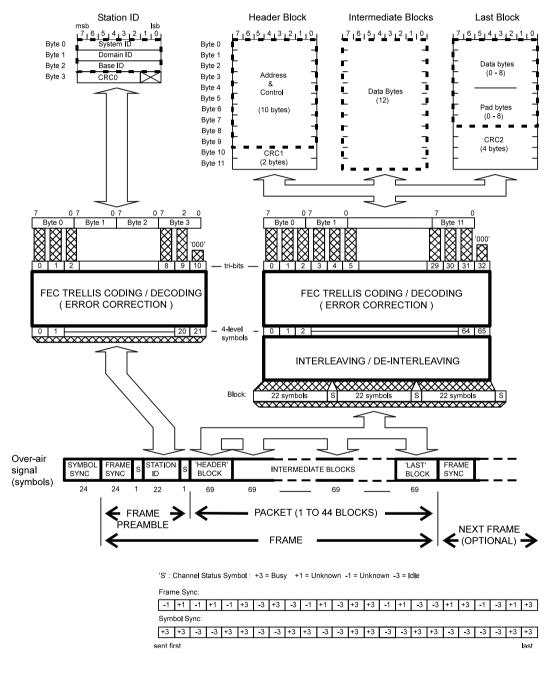
Figure 60 RD-LAP Over Air Signal Format
