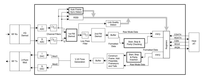
Figure 6 FI-6.x Block Diagram - Two-point Tx with I/Q Rx
