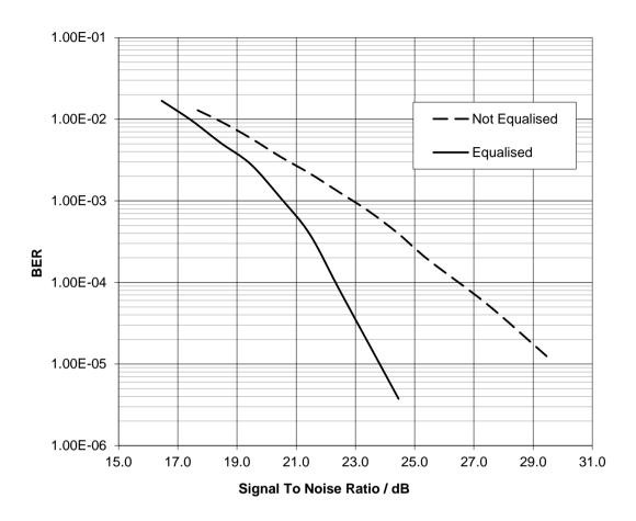
Figure 79 8-FSK Signal-to-Noise Performance, Equalised and Non-Equalised
