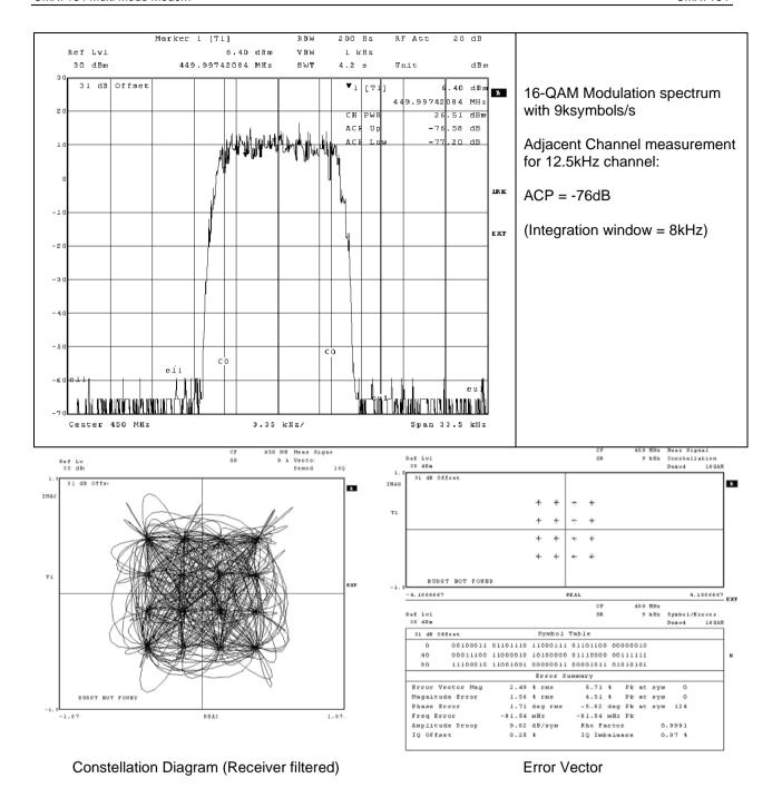
Figure 91 Tx Modulation Spectra (16-QAM), 9ksymbols/s I/Q Modulation into CMX998
