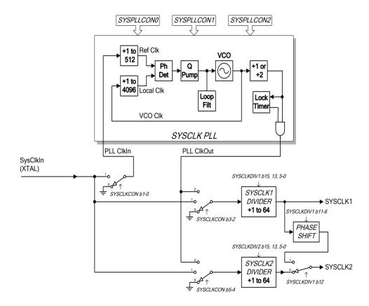
Figure 43 Digital System Clock Generation Schemes
