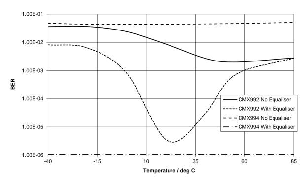
Figure 106 Performance of 64-QAM Equalised Signals with Temperature Variation
