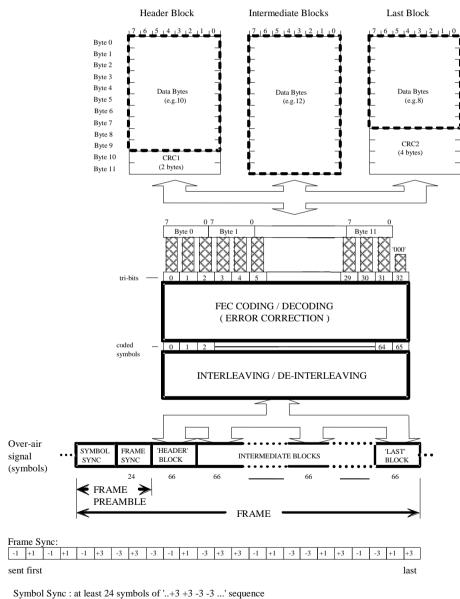
Figure 58 Native Formatted Data Over Air Signal Format
