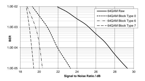
Figure 97 64-QAM Performance with Different Coding Schemes
