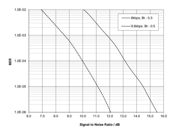
Figure 52 Modem Sensitivity Performance
