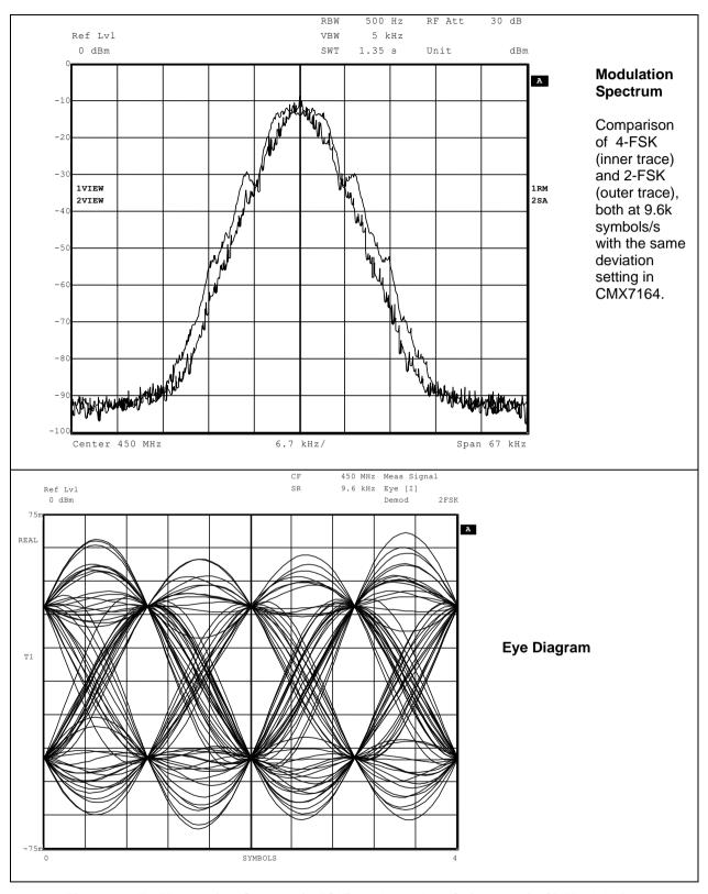
Figure 63 Tx Modulation Spectra (2-FSK), 9.6k symbols/s (9.6kbps), I/Q Modulation
