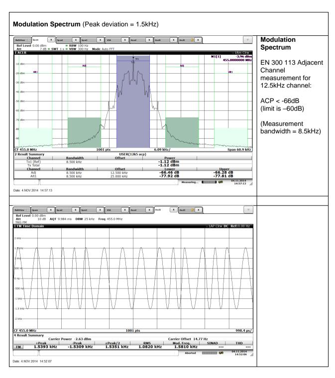
Figure 110 Tx Modulation V.23, 1200bps, I/Q Modulation
