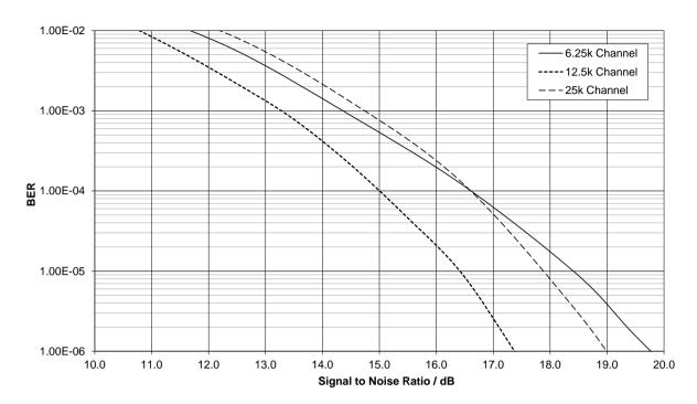
Figure 68 Modem Sensitivity Performance (Root Raised Cosine Pulse Shaping)
