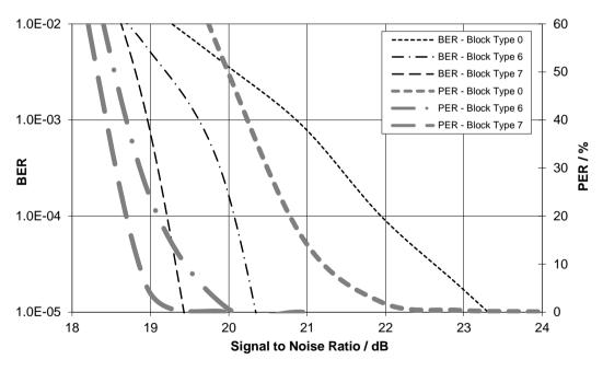
Figure 101 Comparison of BER and PER for 64-QAM Modulation
