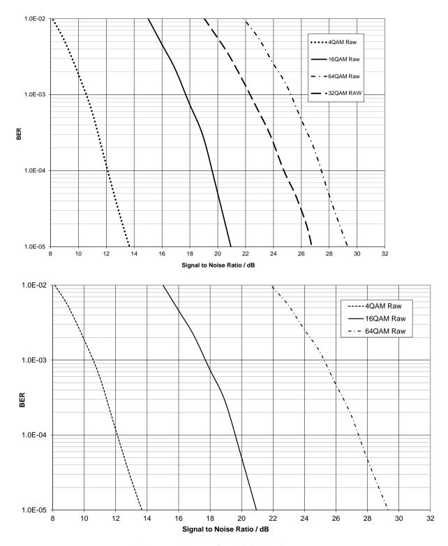
Figure 92 Modem Sensitivity Performance
