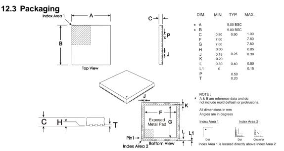
Depending on the method of lead termination at the edge of the package, pull back (L1) may be present.
