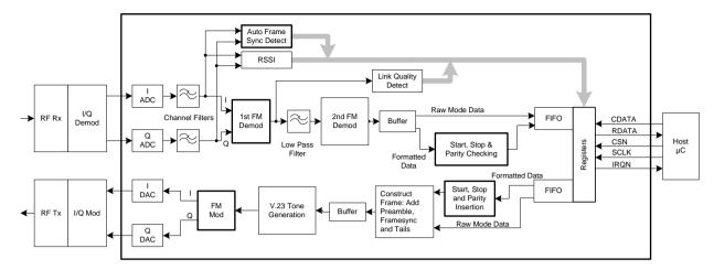
Figure 5 FI-6.x Block Diagram - I/Q Tx and Rx
