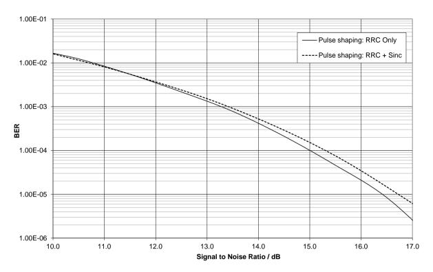
Figure 69 12.5kHz Channel Sensitivity With and Without Sinc Filter Comparison
