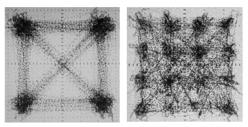
Figure 85 Received 4 and 16-QAM signals, no equalisation
