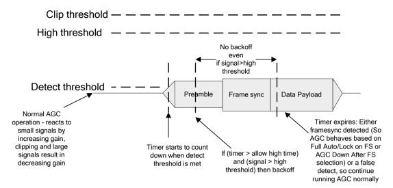
Figure 41 AGC Behaviour During Burst Reception
