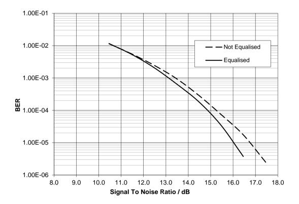
Figure 78 4-FSK Signal-to-Noise Performance, Equalised and Non-Equalised
