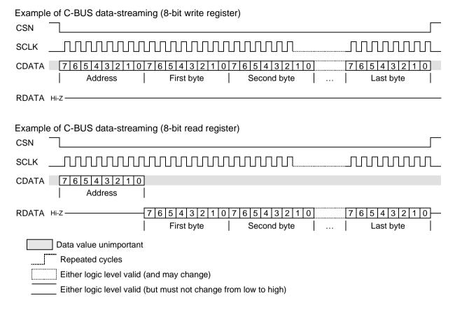
Figure 14 C-BUS Data Streaming Operation
