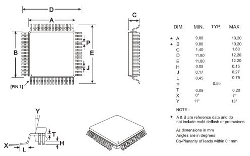
Figure 115 Mechanical Outline of 64-pin LQFP (L9) Order as part no. CMX7164L9
