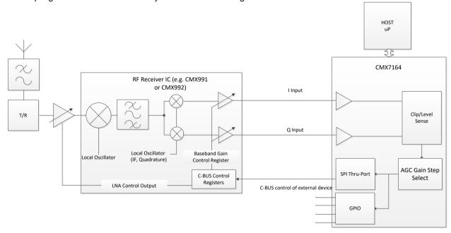
Figure 39 AGC using SPI Thru-Port
