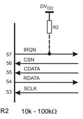
Figure 9 Recommended External Components - C-BUS Interface
