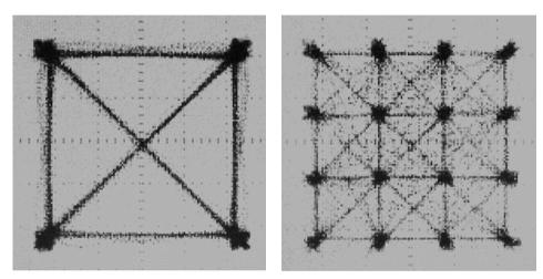
Figure 86 Received 4 and 16-QAM signals with equalisation
