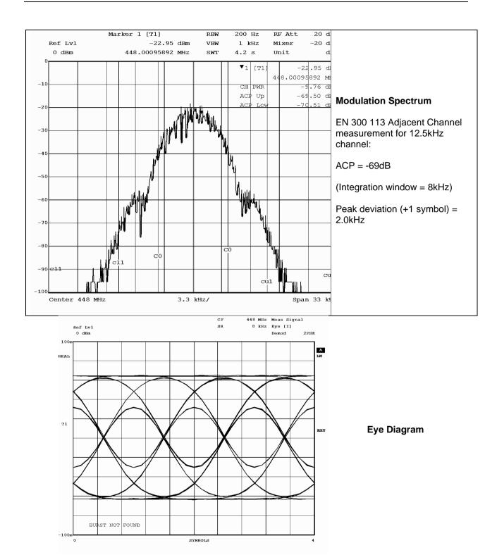
Figure 51 Tx Modulation Spectra (GMSK), 8kbps, BT=0.3 Two-point Modulation
