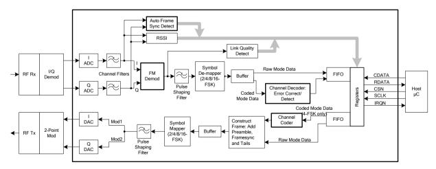
Figure 4 FI-1.x / FI-2.x Block Diagram – two-point Tx with I/Q Rx
