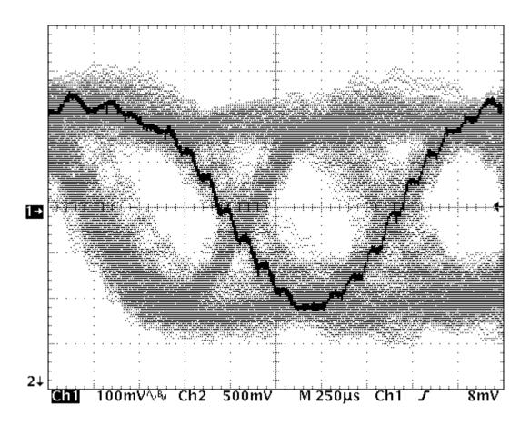
Figure 37 Received Signal (Second FM Demodulator) 7164FI-6.x
