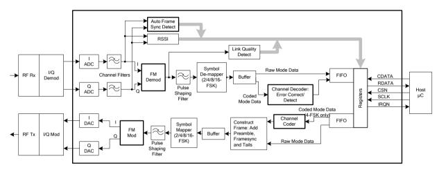
Figure 3 FI-1.x / FI-2.x Block Diagram - I/Q Tx and Rx
