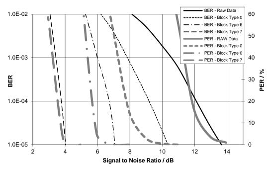
Figure 98 Comparison of BER and PER for 4-QAM Modulation
