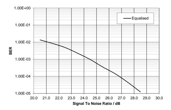
Figure 104 64-QAM Signal-to-Noise Performance, Equalised
