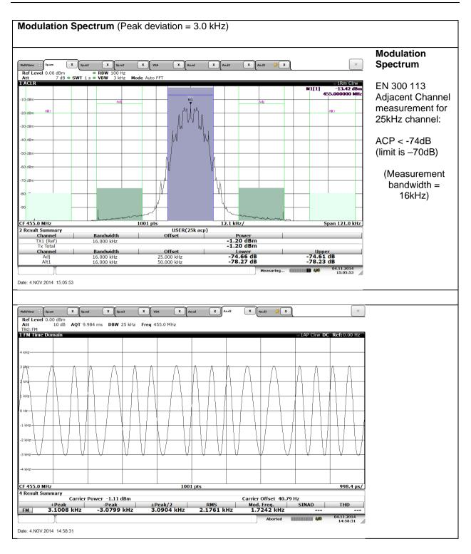
Figure 111 Tx Modulation V.23, 1200bps, I/Q Modulation
