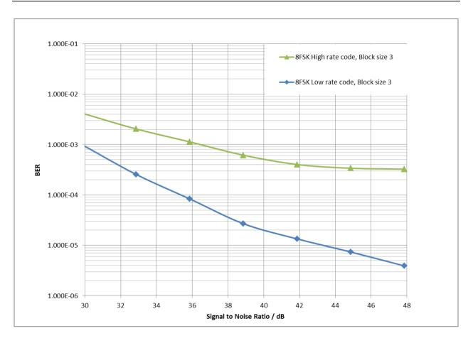
Figure 75 8-FSK Coding Performance in TU50 Fading Channel, 150MHz
