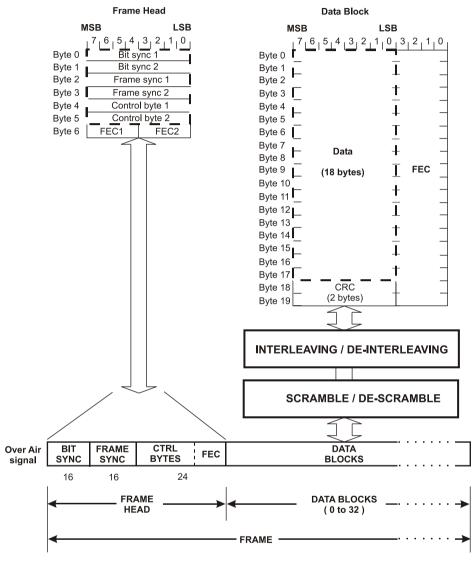
Figure 46 Formatted Data Over Air Signal Format
