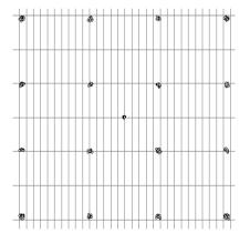
Figure 30 Sample at Symbol Timing with I/Q DC Offset Diagnostic Mode (no frequency error)
