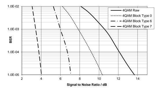
Figure 94 4-QAM Performance with Different Coding Schemes
