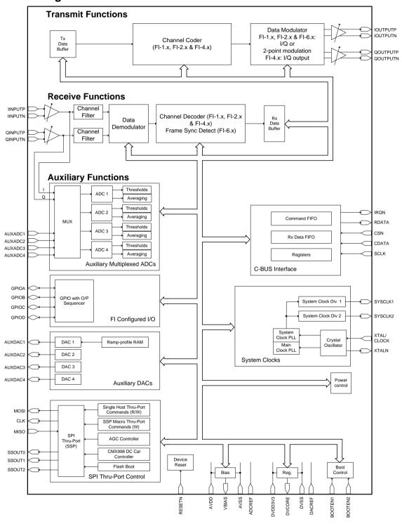
Figure 1 Overall Block Diagram
