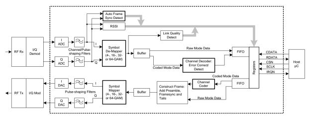
Figure 2 FI-4.x Block Diagram - I/Q Tx and Rx
