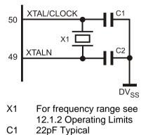
Figure 8 Recommended External Components - Xtal Interface
