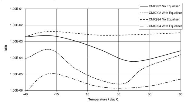
Figure 107 Performance of 16-QAM Equalised Signals with Temperature Variation and Constant Signal-to-Noise Ratio
