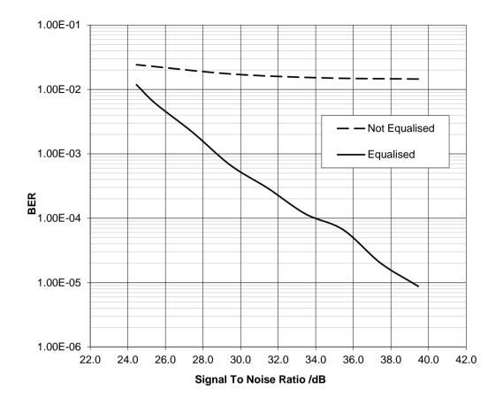
Figure 80 16-FSK Signal-to-Noise Performance, Equalised and Non-Equalised
