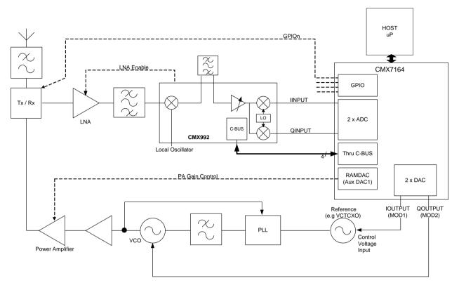
Figure 57 Outline Radio Design (2 or 4-FSK – I/Q in, two-point mod out)
