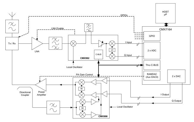
Figure 44 Outline Radio Design (I/Q in/out for GMSK/GFSK)
