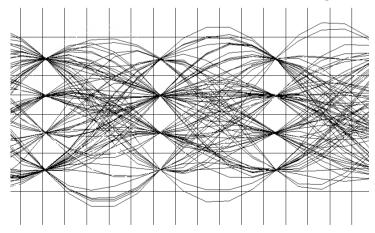
Figure 28 Received Eye Diagram7164 FI-2.x (4-FSK mode)
