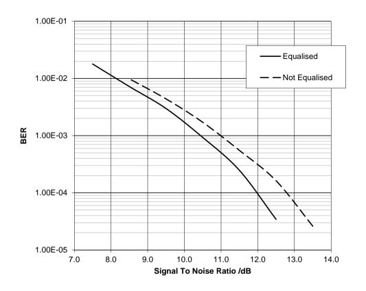
Figure 102 4-QAM Signal-to-Noise Performance, Equalised and Non-Equalised
