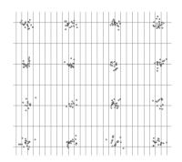
Figure 33 Normalised Constellation (noisy received signal)
