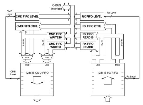
Figure 38 Command and Rx Data FIFOs
