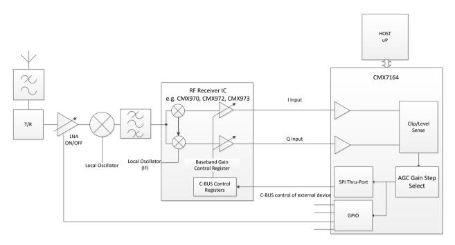
Figure 40 AGC using SPI Thru-Port and external LNA
