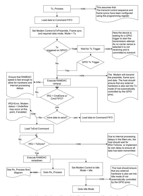
Figure 17 Host Tx Data Flow (No Tx Sequence/Carrier Sense)
