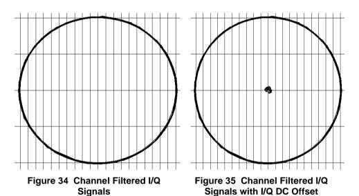
**Note:** The images of receive diagnostic modes shown above are idealised. In practice when using the I Output and Q Output signals to view diagnostics the transitions between constellation point are not instantaneous. Using an analogue oscilloscope is the best way to observe these diagnostic signals.
