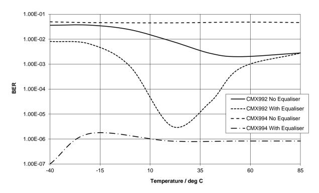
Figure 108 Performance of 64-QAM Equalised Signals with Temperature Variation and Constant Signal-to-Noise Ratio
