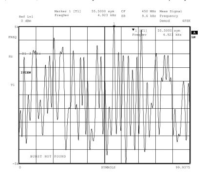
Figure 55 PRBS Waveform (Two-point Modulation)
