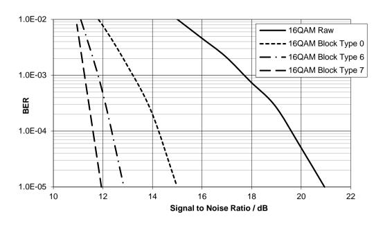
Figure 95 16-QAM Performance with Different Coding Schemes
