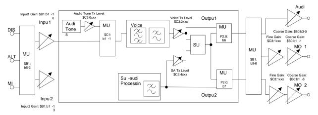
Figure 10 Tx Level Adjustments
