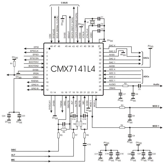
Figure 2 CMX7141 (L4 and Q3) Recommended External Components
