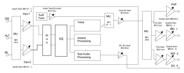
Figure 11 Rx Level Adjustments
