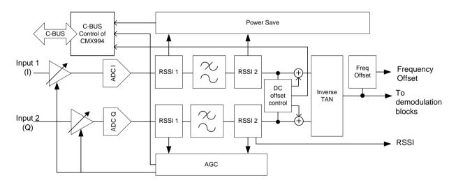
Figure 7 Internal I/Q Processing
