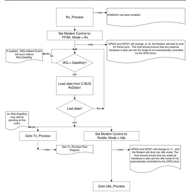
Figure 17 FFSK Rx Data Flow
