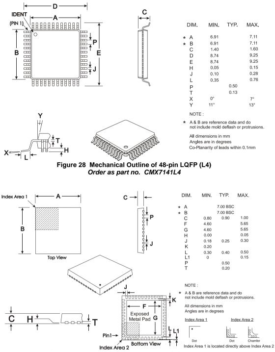
Depending on the method of lead termination at the edge of the package, pull back (L1) may be present.
