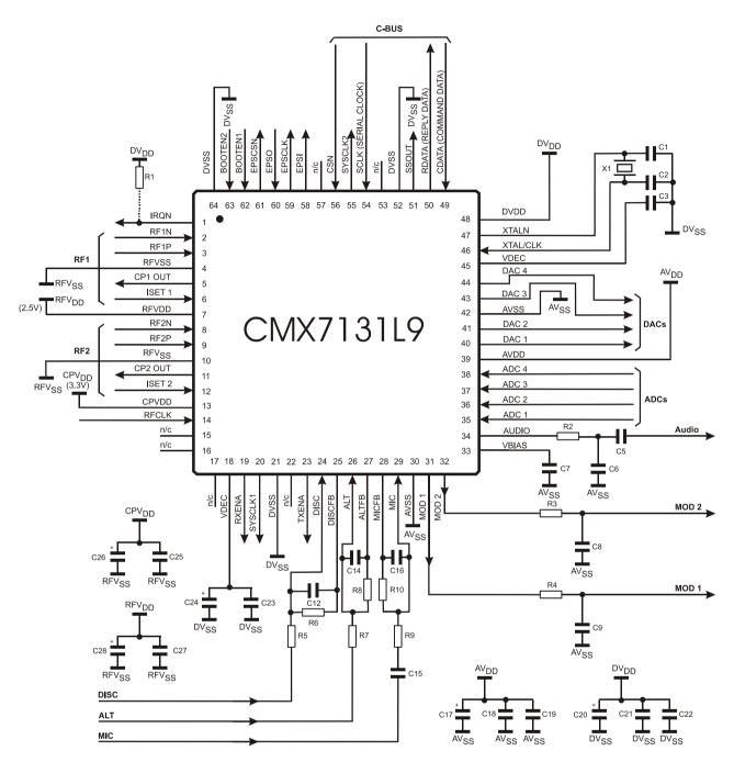
Figure 3 CMX7131 (L9 and Q1) Recommended External Components
