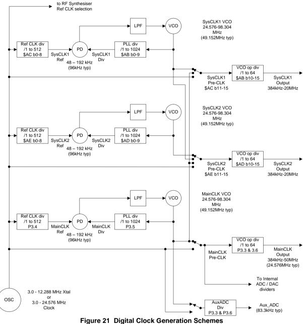
The CMX7131/CMX7141 includes a two-pin crystal oscillator circuit. This can either be configured as an oscillator, as shown in Section 4.2, or the XTAL input can be driven by an externally generated clock. The crystal (Xtal) source frequency can go up to 12.288MHz (clock source frequency up to 24.576MHz), but a 19.2MHz oscillator is assumed by default for the functionality provided in the CMX7131/CMX7141.
