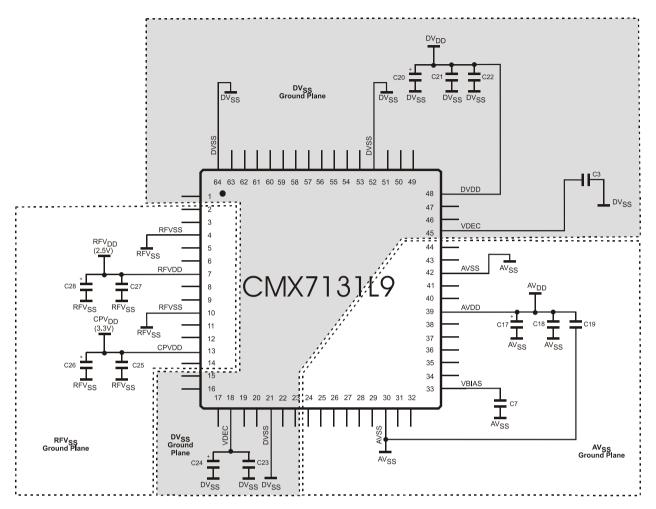
Figure 5 CMX7131 (L9/Q1) Power Supply and De-coupling Component Values as per Figure 3
