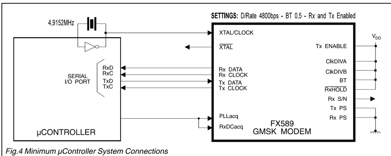
Fig.4 Minimum  $\mu$ Controller System Connections
