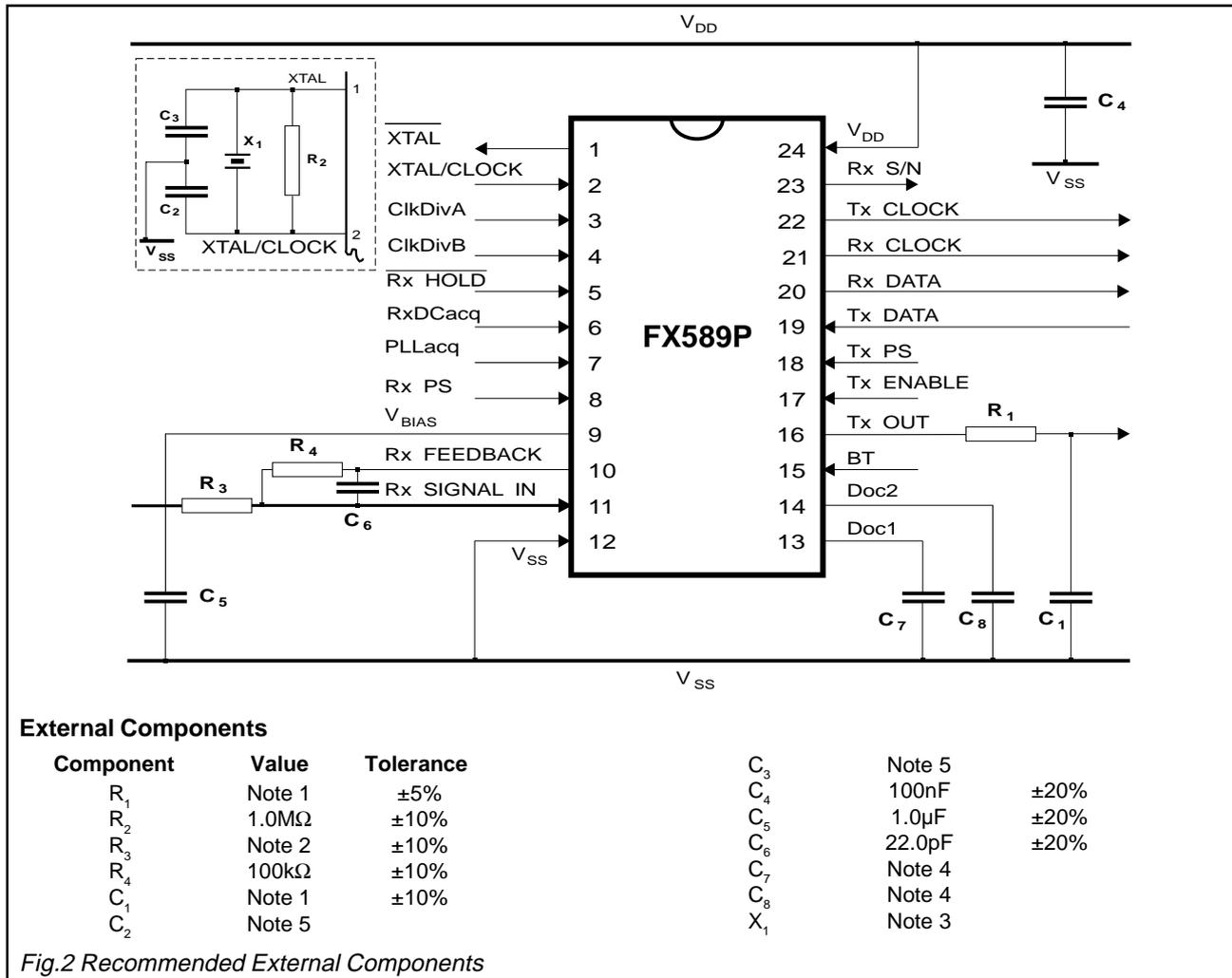
Fig.2 Recommended External Components
