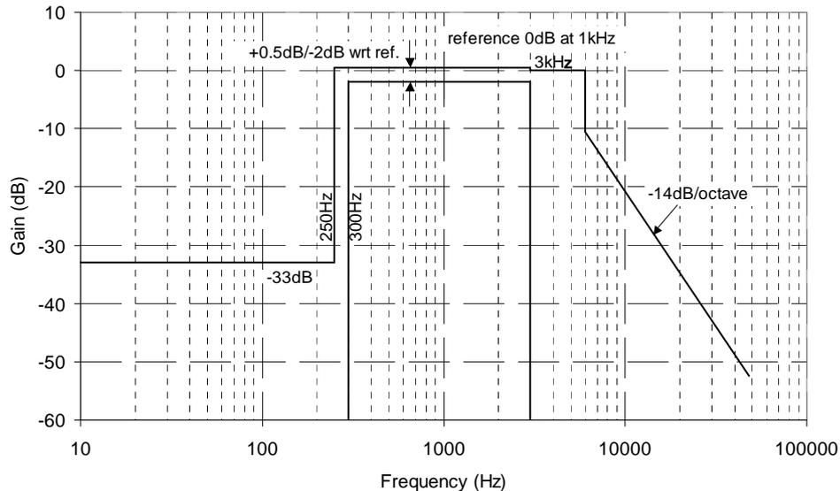
**Figure 8 25kHz Channel Audio Filter Response Template**
