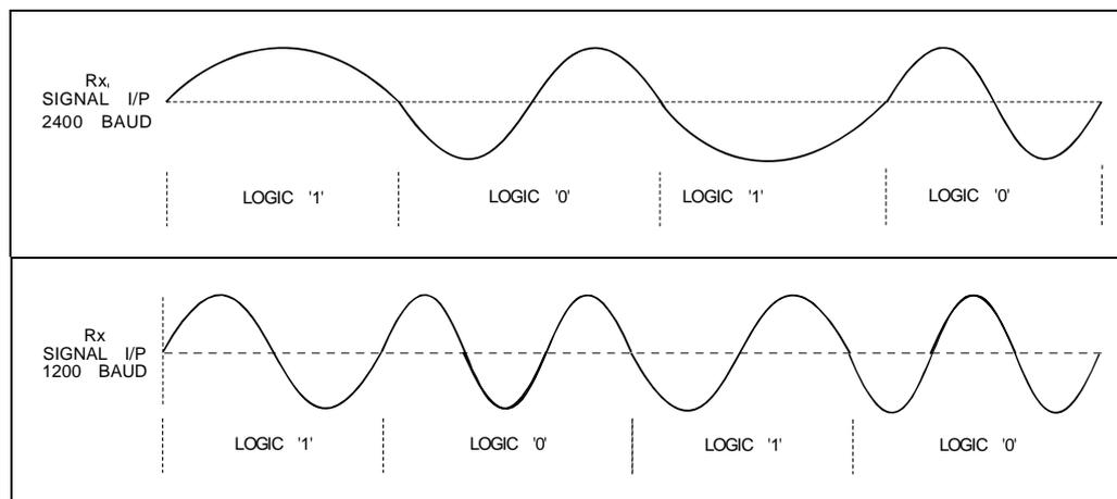
**Figure 11 Modulating Waveforms for 1200 and 2400 Baud FFSK/MSK Signals**
