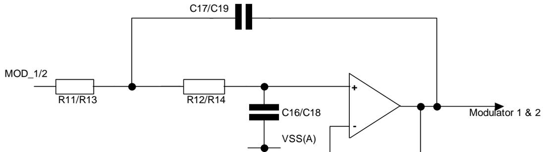
**Figure 4 Modulator output components to achieve  $-100\text{dB/decade}$  roll-off**
