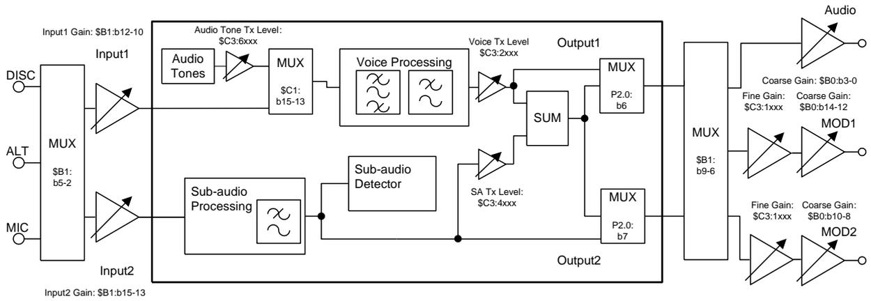
Figure 15 Tx Level Adjustments
