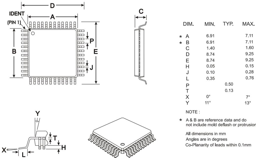
**Figure 34 Mechanical Outline of 48-pin LQFP (L4)**
