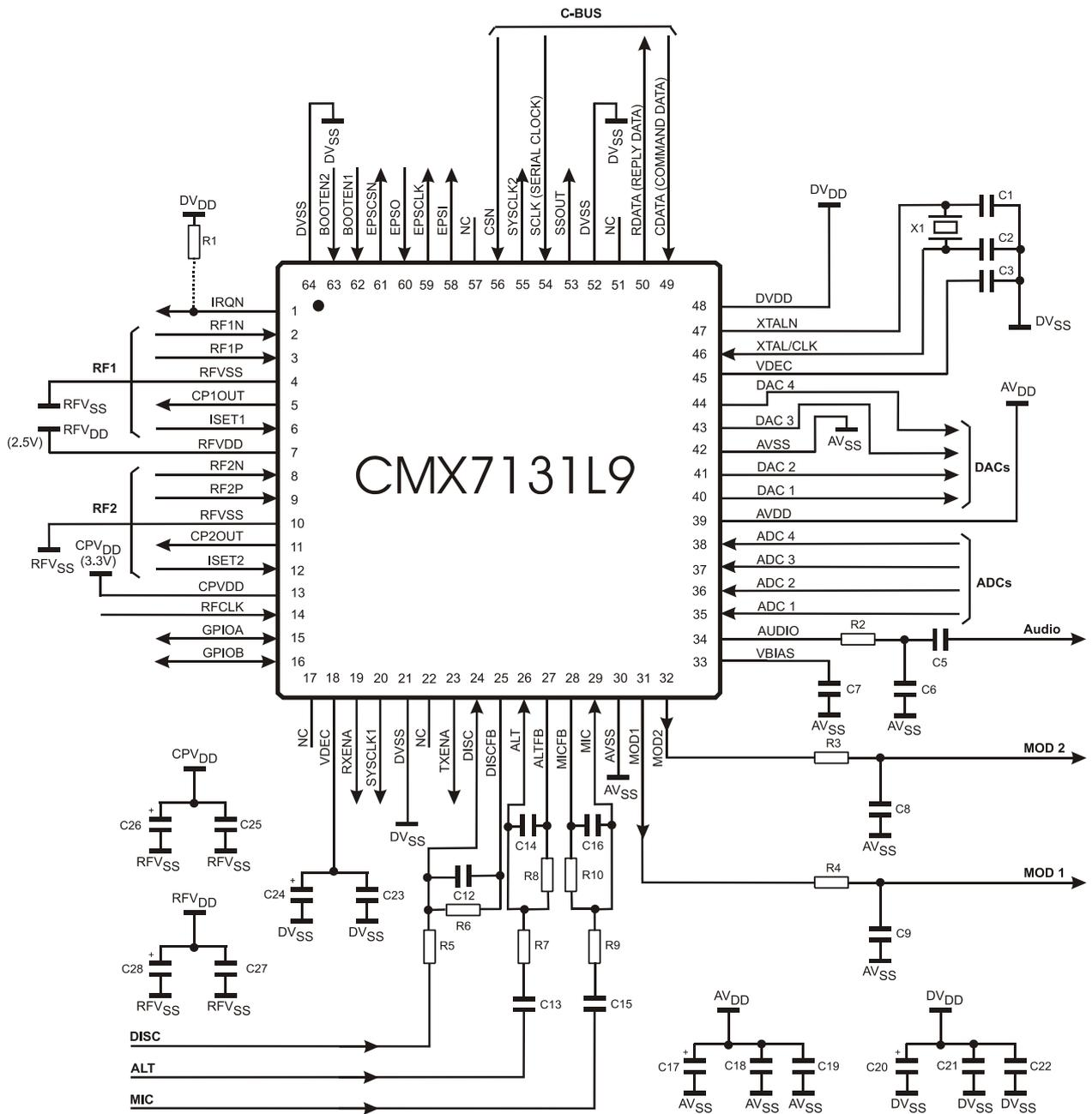
Figure 3 CMX7131 (L9 and Q1) Recommended External Components
