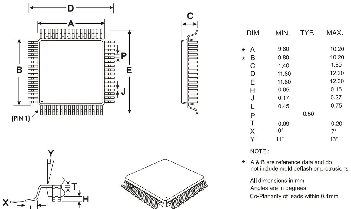
**Figure 33 Mechanical Outline of 64-pin LQFP (L9)**
