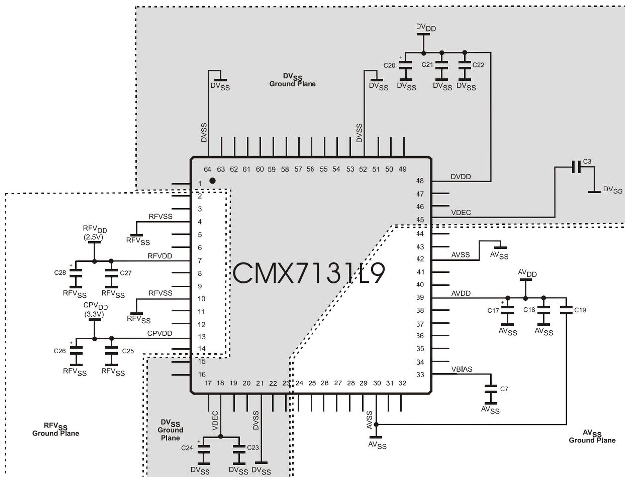
**Figure 5 CMX7131 (L9/Q1) Power Supply and De-coupling**
