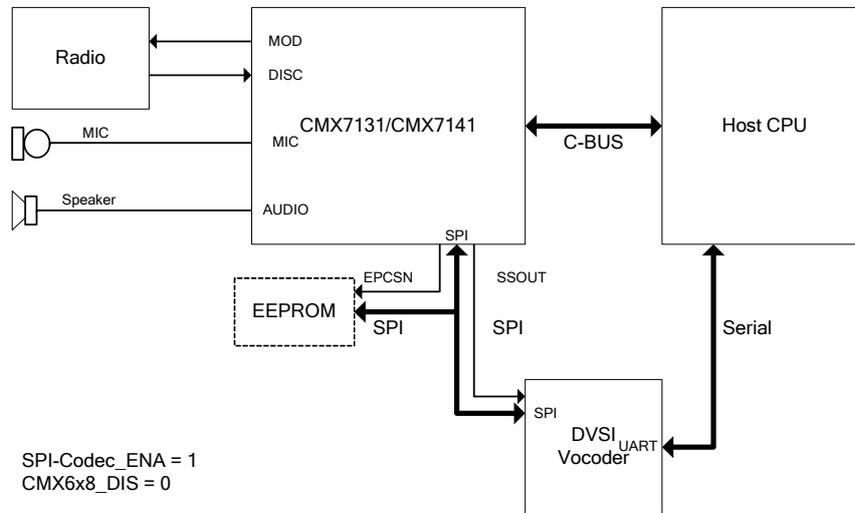
**Figure 8 DVSI Vocoder Connection**
