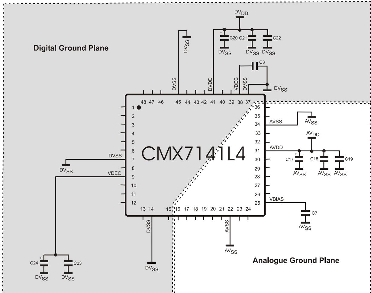
Figure 4 CMX7141 (L4/Q3) Power Supply and De-coupling
