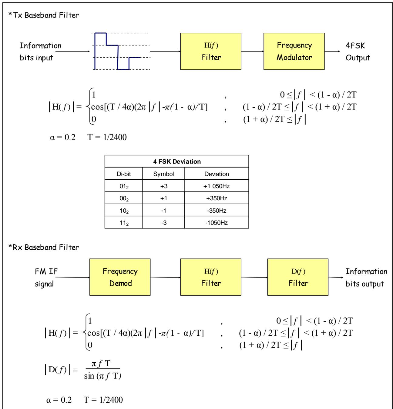
**Figure 12 dPMR Modulation Characteristics**
