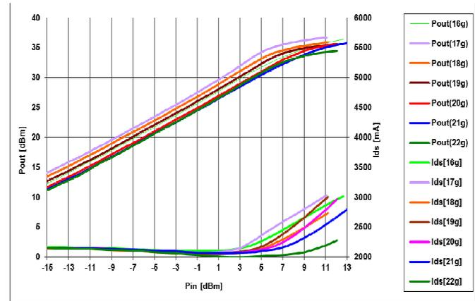
Pout[dBm], and Ids[mA] vs. Input power [dBm]
