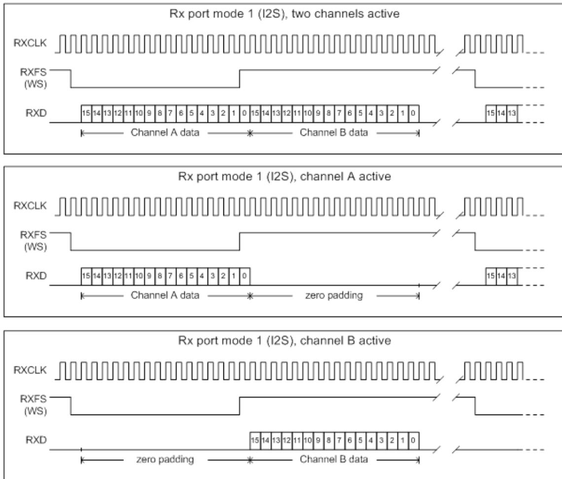
**Figure 6 Rx I<sup>2</sup>S Timing (identical for Tx)**
