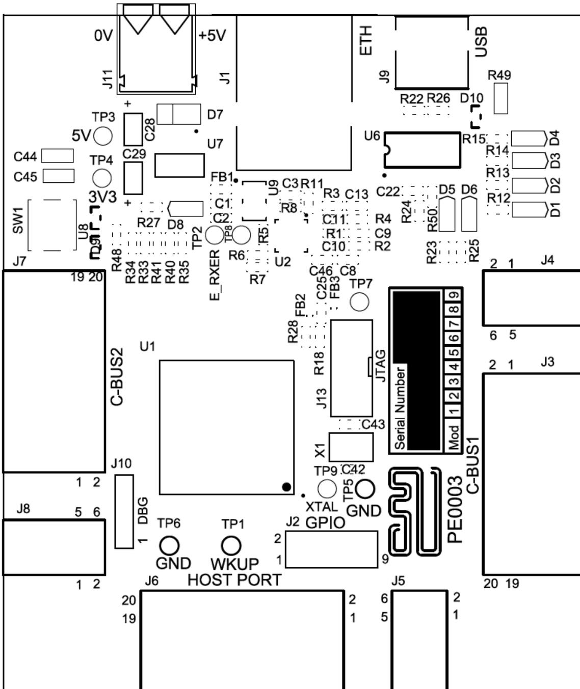
Figure 2 PE0003 Interface Card Top Layout
